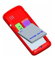
**Install:** (1)Match the metal contacts of battery separately with the battery compartment metal contacts, and put the battery base into the slot;
