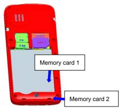
Keep the metallic face of a memory card downward, and slide it gently to the position of Memory card 1.
