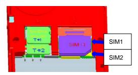
Keep the metallic face of a SIM card downward, and slide it gently to the position of SIM 1.
