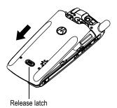
Slide USIM card door to the left and lift open.
