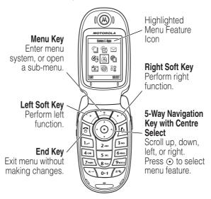
Press  $\textcircled{\odot}$  to scroll to and highlight a menu feature icon in the main menu. Press **SELECT** ( $\textcircled{\circ}$ ) or  $\textcircled{\circ}$  to select the highlighted menu feature.
