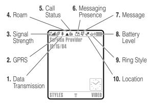
Data Transmission Indicator – Shows connection and data transmission status. The Bluetooth<sup>®</sup> wireless connection indicator ≱ shows when a Bluetooth connection is active. Other indicators can include:
