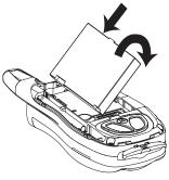
3 To replace the battery door, locate the tabs on the battery door and the slots in the phone.
