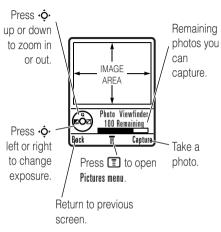
**Note:** Adjusting the exposure affects the brightness of both the viewfinder display and the captured photo.
