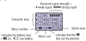
Following some operations the display will automatically clear after three seconds or after pressing any key except ...
