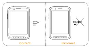
① Note Make sure to align the connector as indicated in the image. Otherwise, the charging connector will be damaged and the battery will not be charged.
