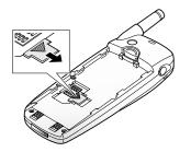
4. Insert the SIM card under the two tabs, ensuring that the cut corner is lower right and the gold contacts of the card face into the phone.
