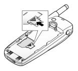
6. Place the battery back on the phone. Slide the battery up towards the catch until it locks into place. Make sure that the battery is properly installed before switching on the phone.
