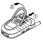
To install, fit the hooks into the notches on the front of the phone and press down firmly until it snaps into place.
