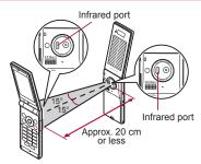
Face the Infrared ports of the receiver's and sender's FOMA terminal each other and set the distance between them to approximately 20 cm or less as shown.
