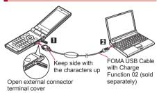
Insert the FOMA side of the FOMA **USB Cable with Charge Function 02** (sold separately) into the external connector terminal on the FOMA terminal ( 11).
