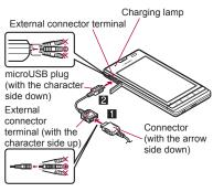
When inserting the AC adapter power plug into an outlet or inserting the DC adapter power plug into a car cigarette lighter socket, charging lamp illuminates and charging starts
