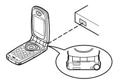
When using the infrared modem function for executing data transmission, align the infrared port with each other.
