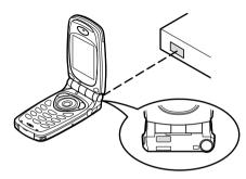
When using the infrared modem function for executing data transmission, align the infrared port with each other
