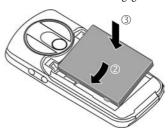
To remove, press the retaining tab on the side of the battery, then lift the battery out.  Place the battery cover on the phone slightly off centre and then slide it until it clicks into place.
