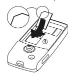
Insert the battery sideways into the phone <sup>(4)</sup>, then press it downwards <sup>(5)</sup> until it clicks into position.
