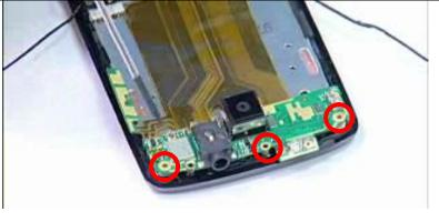
Put the Rigid flex board on the bezel.
