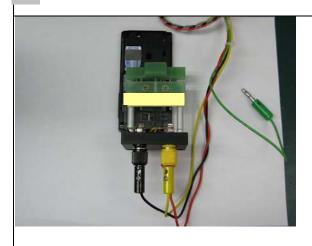
3. Install jig to device (the photo is for reference only)
