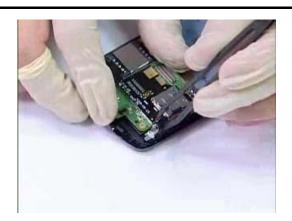
Assemble the vibrator on bezel as shown
