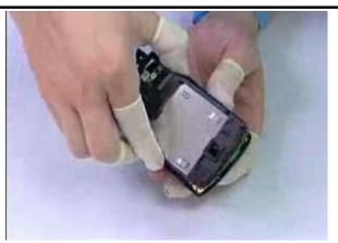
Combine the housing with bezel Caution: Make sure the Main camera is inserted correctly
