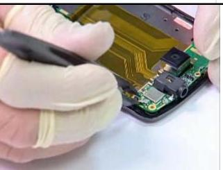
Disconnect the GPS coaxial cable from Rigid flex board as shown.
