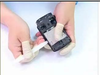
Insert the flat plastic stick between the Housing and Bezel to separate the Housing
