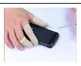
Insert the stylus into the slot
