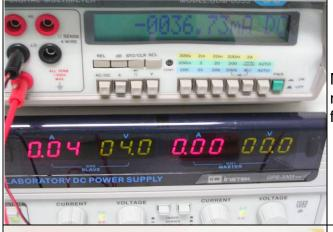
Measure Idle mode current. Current value must under 50mA, if over, it means M/B failed, please replace M/B for repair.
