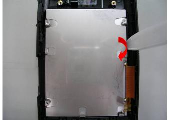
Use plastic stick to take LCM module with holder out.
