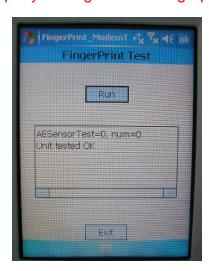
**Step 6:** Tap Exit button to leave Fingerprint Test function and then tap Modem Test button.
