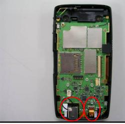
Place RJ11 connector into bezel and connect key pad cable.
