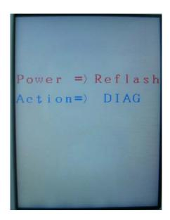
**Step 4**: After finishing the re-flash process, please press action button and then choice function test to check checksum.
