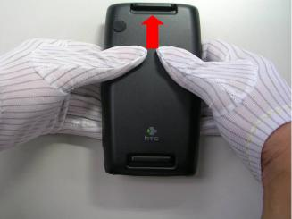
Press battery cover with your two thumbs to move battery cover forward.
