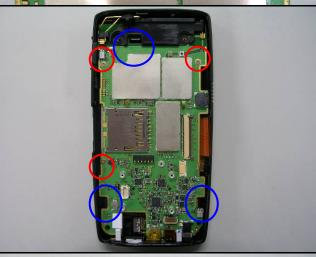
Place main board into bezel and ensure three hooks are locked completely then fasten three screws.
