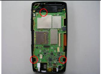
Use plastic stick to loosen three hooks and then take main board out from bezel.
