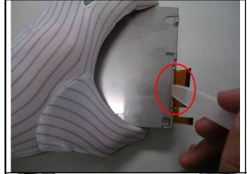
Use plastic stick to press LCM module and then separate LCM module from holder
