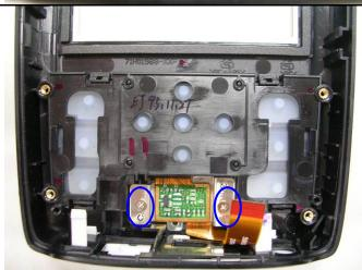
Place finger print module into the bezel and then fasten two screws.
