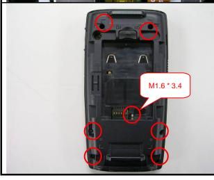
Combine bezel with housing and then fasten six screws (M1.6\*6 mm) and one screw (M1.6\*3.4).
