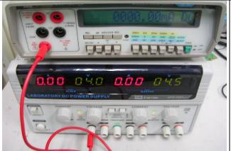
Connect cable (D) to positive polarity of power supply (A) and current meter (B).
