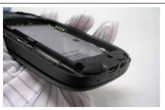
Using the flat stick and move along the gap of the unit.
