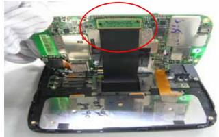
Lift up the main board, release the LCM FPC and take out the MB
