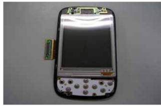
Fasten 4 screws of RF board to display bottom cover
