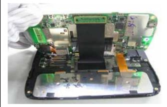
Pull out the slider and connect LCM FPC into MB Then stick LCM FPC with adhesive tape, plus one tape to fix LCM FPC
