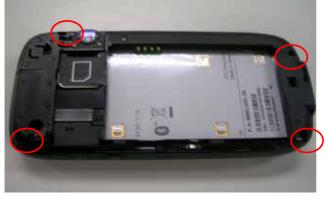
Fasten 4 screws on rear side 72H01691H-00M
