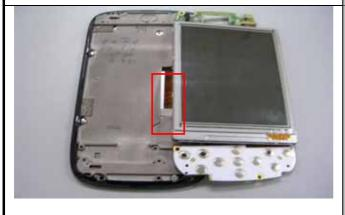
Put the RF board FPC to pass through slider hole
