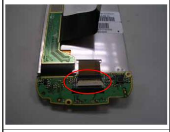
Release LCM FPC, separate RF board from LCM
