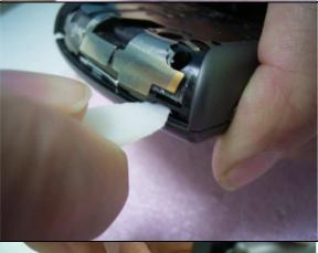
Push up to unlock hook of the antenna cover (Step2)
