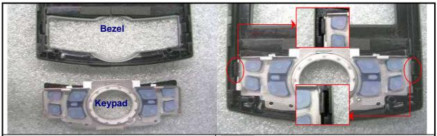
Assemble the Keypad on the Bezel; please 100% make sure that the hooks of the Bezel are hooking the Keypad properly. **Keypad:** 74H00772-00P/Q'ty:1. **Bezel:** 74H00762-01M/Q'ty:1 **[Option]**.
