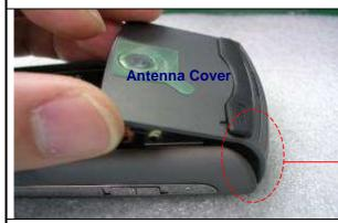
• Assemble Antenna Cover to Housing.
