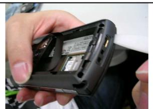
Move the stick slightly around the device to unlock the hook (Step4)
