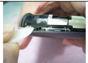
Insert a plastic stick under the housing and push up to unlock hook of the antenna cover (Step1)
