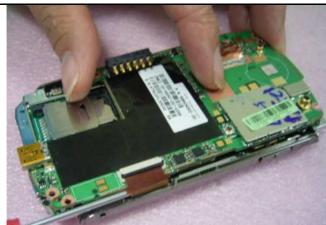
Open LCM FPC gate and pull off the LCM FPC
