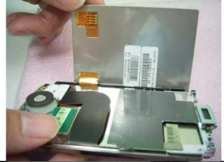
Peel off the LCM from the chassis
