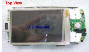
Assemble the **LCD Module** to the Chassis, and insert the LCD FPC through into the Chassis and connect to M/B properly.
