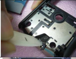
Use a plastic stick to push speaker out of the housing to separate
