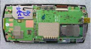
Assemble the M/B to the Bezel, and insert the edge of the Receiver frame of the Chassis into the Bezel properly.
