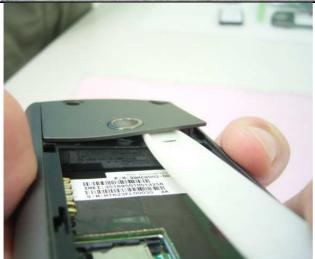
Insert a plastic stick into the beside the camera lens to unlock the antenna cover
