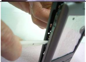
Move the stick slightly around the device to unlock the hook (Step3)
