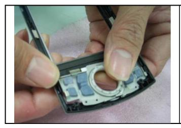
Pull hook of the bezel and push the keypad out of the bezel
