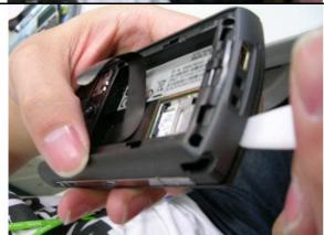
Move the stick slightly around the device to unlock the hook (Step5)
