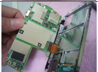
Open the switch board FPC gate and pull off the switch board FPC to separate the chassis and main board
