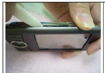
Insert a plastic stick into space between chassis and bezel to unlock chassis and bezel
