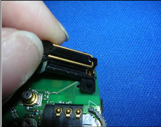
Take out the antenna module from the main board
