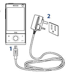
Charging is indicated by a "breathing" white light around the Navigation Control. As the battery is being charged while the power is on, a charging icon so also appears in the title bar of the Home screen. After the battery has been fully charged, the Navigation Control LED shows a solid white light and a full battery icon the appears in the title bar of the Home screen.
