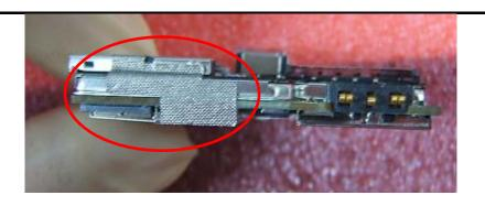
PASTE A CONDUCTIVE FABRIC (72H02845-00M) AT THE LOCATION INDICATED.
