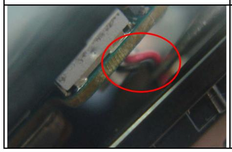
NOTE: USE TWEEZERS TO KEEP THE POSITION OF THE SPEAKER WIRES LOWER THAN THE MAIN BOARD AND KEEP AWAY FROM THE CONNECTOR TO PREVENT THE WIRES BEING PRESSED DURING ASSEMBLY.
