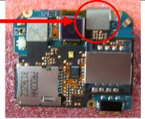
PASTE A CONDUCTIVE FABRIC (76H02985-00M) AT THE LOCATION INDICATED.
