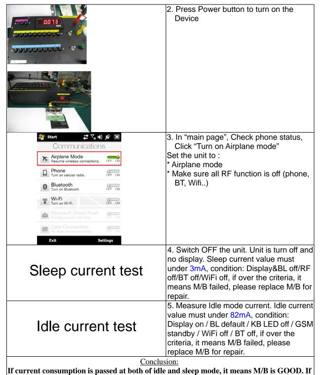
there is any item FAILED at idle or sleep mode, it means M/B is failed, please replace M/B for repair.
