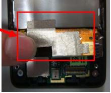
STICK A CONDUCTIVE FABRIC (72H02749-00M) TO THE LCD FPC AS SHOWN
