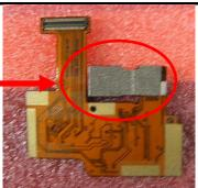
CONNECT THE MAIN CAMERA TO SIM FPC AND STICK THE CONDUCTIVE FABRIC ON IT.
