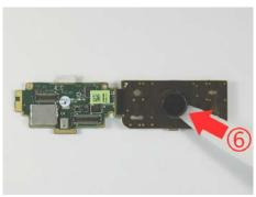
CONTINUE ABOVE STEP AND FOLLOW THE ARROWS DIRECTION TO SEPARATE THE NAVI KEY CAP AND THE FPC.
