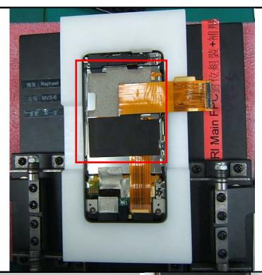
PASTE 2 CONDUCTIVE FABRICS (72H02854-00M & 72H02855-00M) AT THE LOCATION INDICATED.
