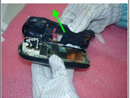
After ALL the hooks around the perimeter of the unit, separate the Rear Housing of the unit as shown in the picture.
