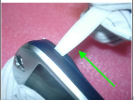
Continue sliding the plastic tools along the unit's Up side and stop before the Infrared port.
