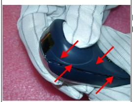
Push the rear housing and gently close it into bezel, the same method apply along the unit.
