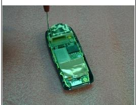
Remove one screw located at the top left side of unit as shown on figure.
