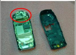
Bezel with Mainboard parts, rear housing.
