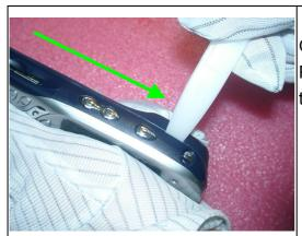
Once the first hook has been released, slide the Plastic Tool along the gap of the unit to unlock the rest of the hooks.
