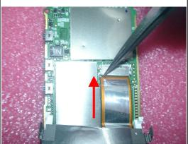
Use Tweezers to push the first side of the connector cover frontward.
