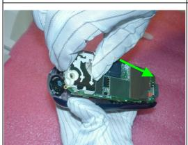
Then pulling leftward the Mainboard to separate the Mainboard with the Bezel.
