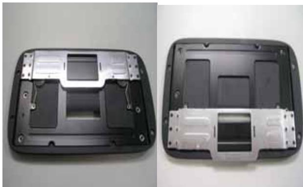
Assemble slider and fasten 6 screws
