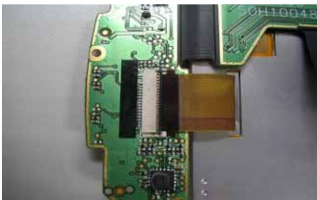
Assemble LCM and connect its FPC into RF board
