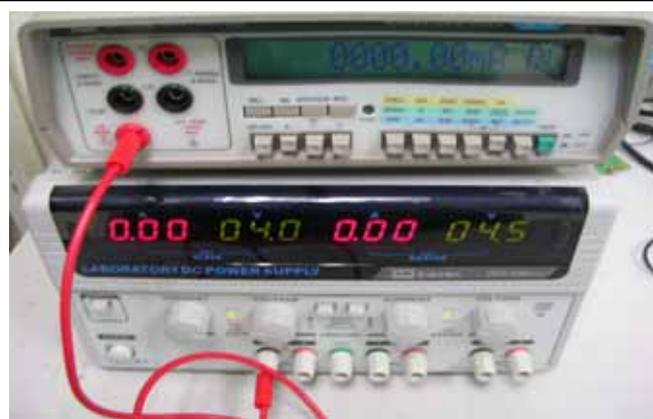
3. Connect cable (C) to positive polarity of power supply (A) and current meter (B)
