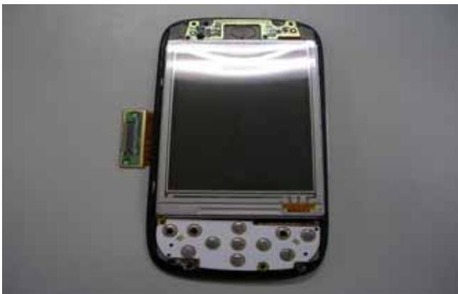
Fasten 4 screws of RF board to display bottom cover
