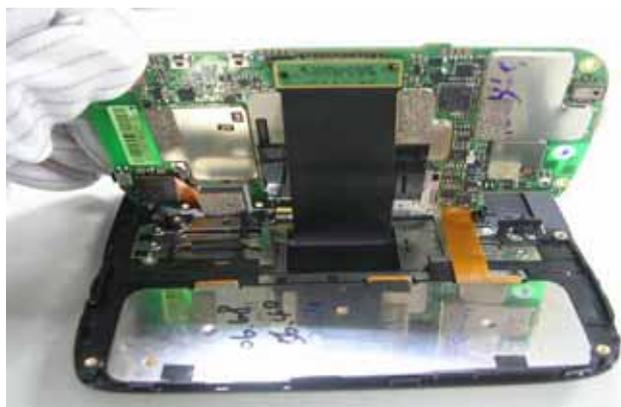
Pull out the slider and connect LCM FPC into MB
