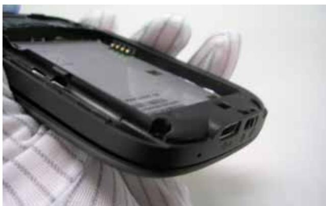
Using the flat stick and move along the gap of the unit.
