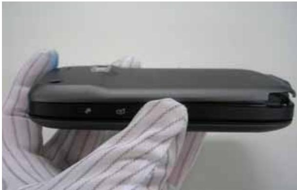
Assemble battery cover and lock it into position
