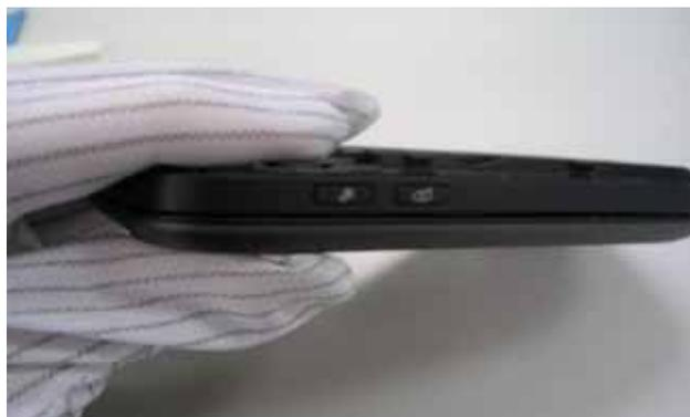
Check each button is assembly properly into its position
