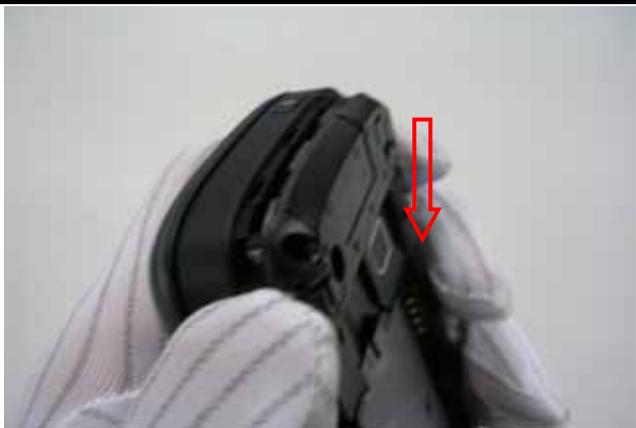
Assemble antenna and speaker module starting from its right lower part
