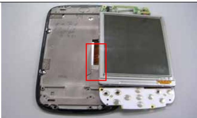
Put the RF board FPC to pass through slider hole
