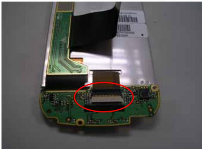
Release LCM FPC, separate RF board from LCM
