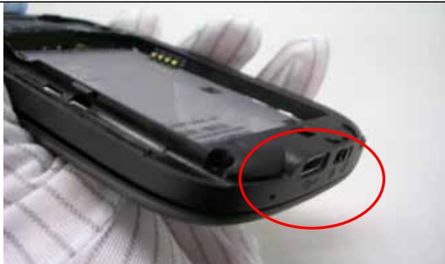
Then assemble MB into housing starting from its USB connector
