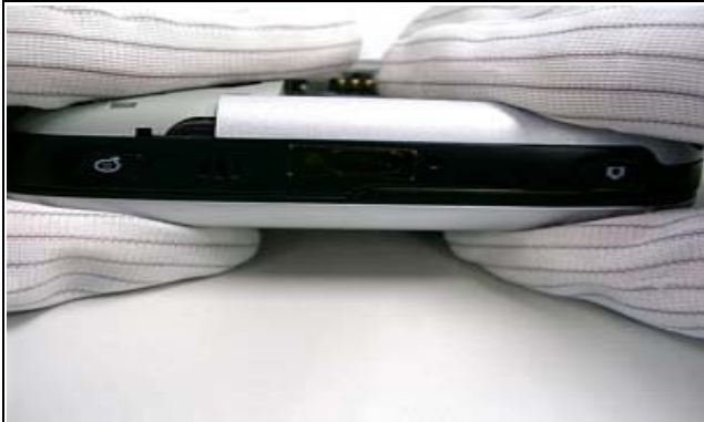
Use finger and thumb to press the hook
