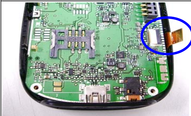
Disconnect keyboard FPC cable
