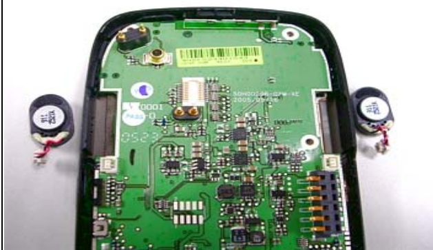
Both side speakers are removed
