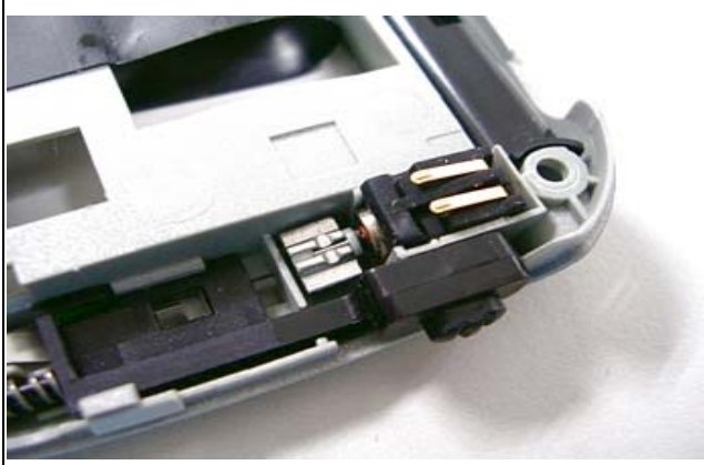
Assembly Vibrator to keypad housing
