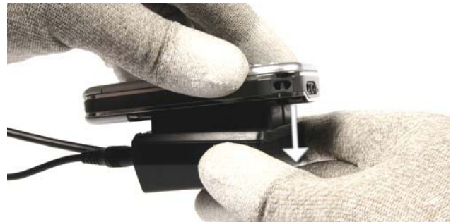
Now, push down the bottom side of the phone, do not use too much force.
