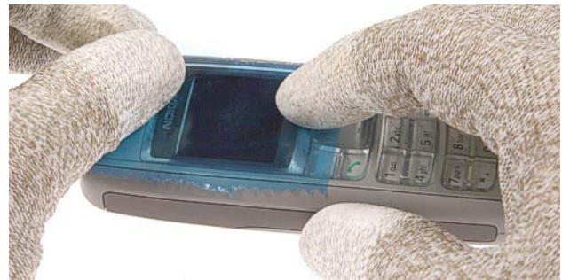
2.) Protect the window with a film.
