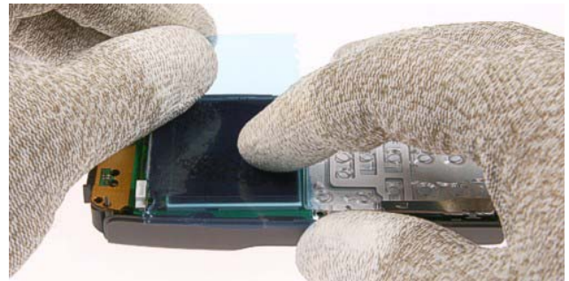
12.) Protect the LCD Module with a film.
