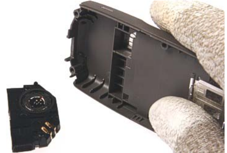
18.) The Antenna IHF Assy drops out when turning the D-Cover Assy .
