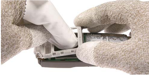
9.) Lift the LCD Shielding while pressing on the LCD Module with a clean cloth carefully.
