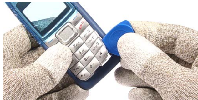
6.) Use SRT-6 to remove the Keymat and protect the inner side of the window with a film.
