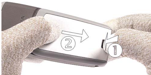
3.) Press the Release Button and remove the B-Cover .
