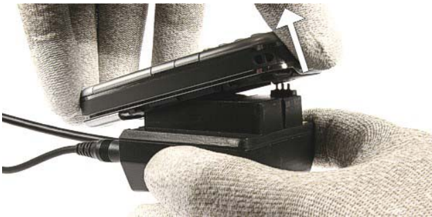
When removing the phone, always start from the bottom side of the unit.
