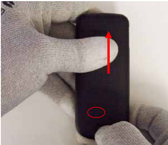
1) Press the release button and slide the B-cover upwards.
