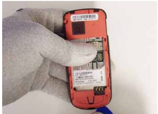
4) Insert the SRT-6 at the bottom of the phone and work around the edges.
