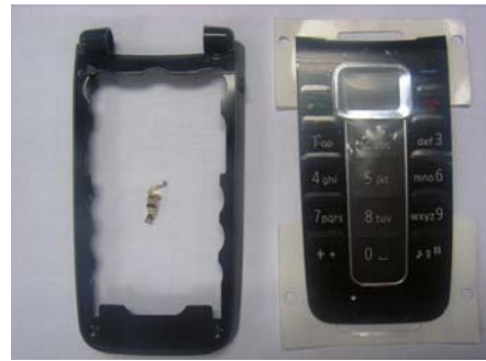
26. Key pad removed.
