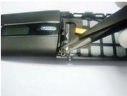
21. Use the tweezers to remove the hinge spring.
