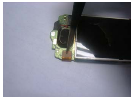
38. Disassemble the BTB Connector of sub LCM - 1.
