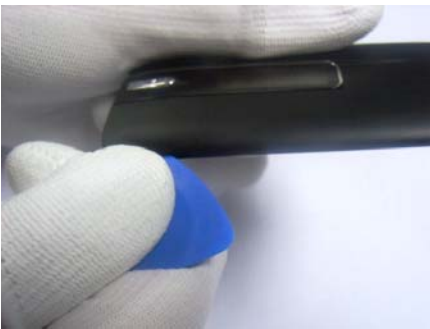
27. Insert the pick into gap and slide along edge to separate housing tabs - 1.
