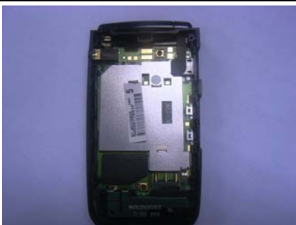
23. MB assembly completed.
