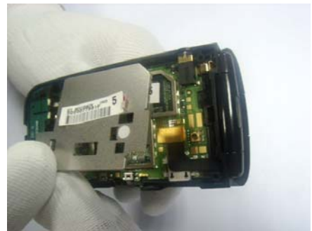
22. Assemble shielding case on MB.
