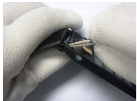
22. Push open the hinge cam by tweezers to separate Housing.
