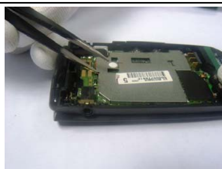
12. Remove the shielding case.
