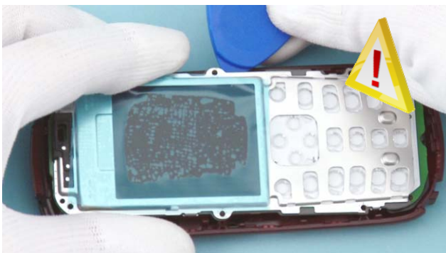
9) Use the SRT-6 to carefully lift up the LIGHT SWAP MODULE.
