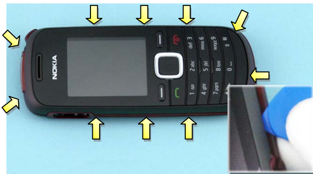
5) Use the SRT-6 to detach the A-COVER. Slide the SRT-6 along the cover edge to release the 10 clips.
