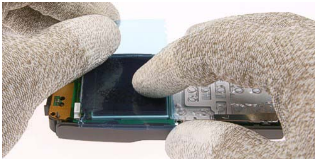
11.) Protect the LCD Module with a film.
