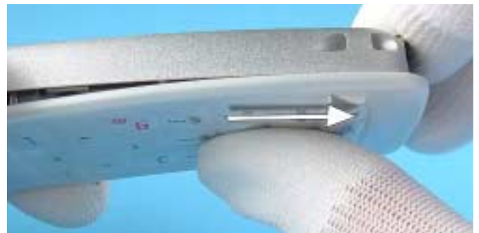
6.) Shift the A-Face Assy from the B-Cover as shown in the picture.
