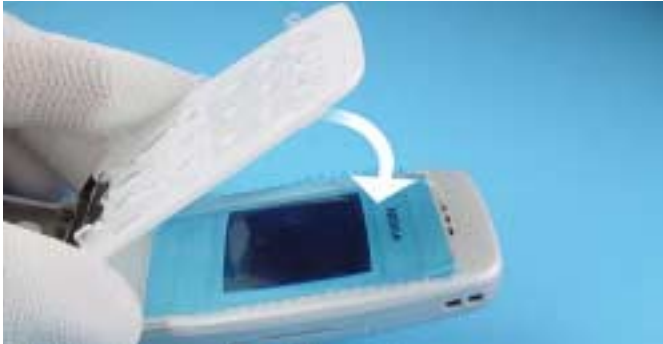
7.) Fold the A-Face Assy as shown in the picture.
