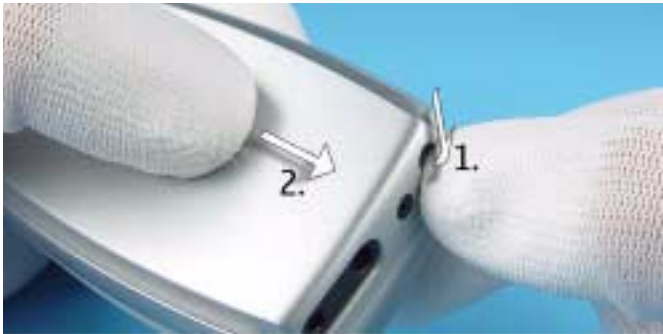
1.) Push down the Release Button before pulling the Battery Cover.
