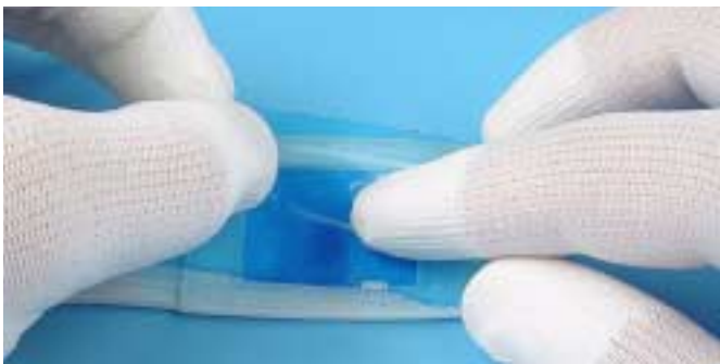
9.) Protect the inner side of the Window with a plastic film.
