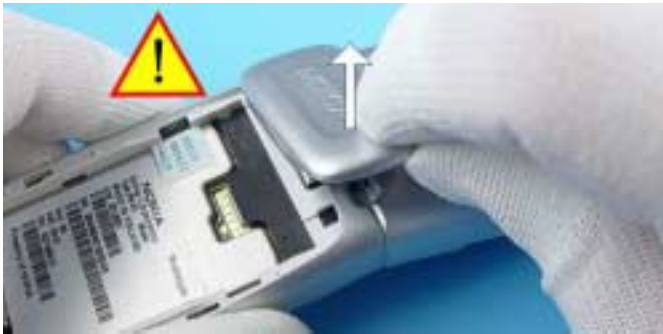
3.) The Backplate is attached to the Hinge Spring with two adhesive tapes. To avoid the snaps from breaking it is important that the Backplate is at first lifted on the right side referring to the "NOKIA" logo.
