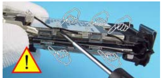
19.) Note the exactly position when laying the Coax Cable during assembly.
