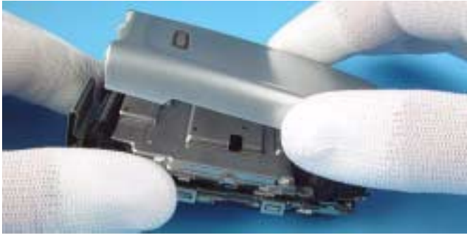
13.) ...and the B-Cover Upper Block can be removed.
