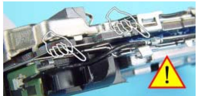
17.) Placement of the Coax Cable in the IHF Antenna Chamber.
