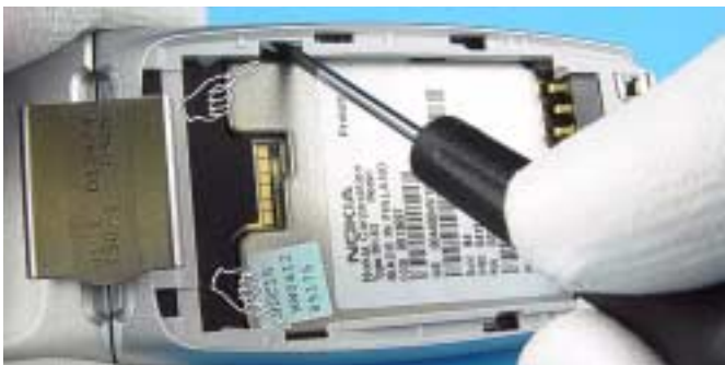
5.) A-Face Assy is attached with snaps to the B-Cover Lower Block. Release the two snaps first.
