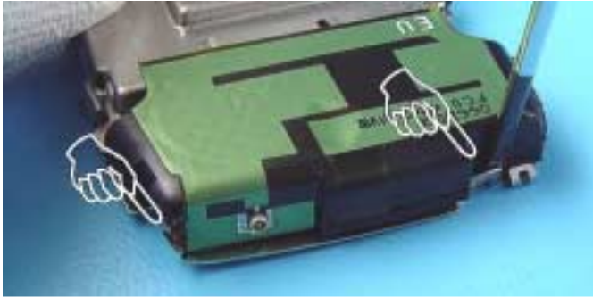
28.) Unlock the snaps before removing the IHF Antenna Chamber.
