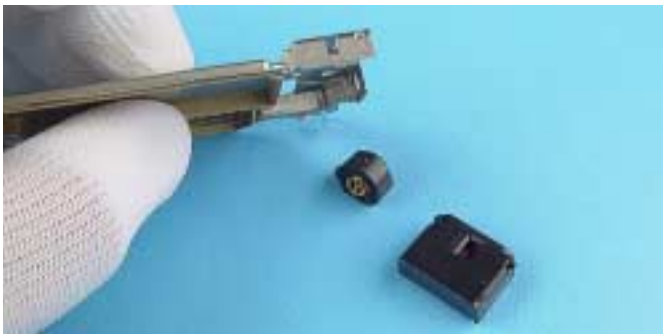
38.) System Connector and Microphone drop out when turning the Shielding Can.
