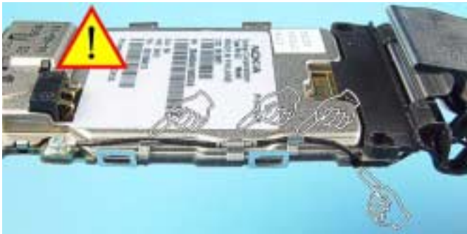
14.) Placement of the Coax Cable in the Lower Block.
