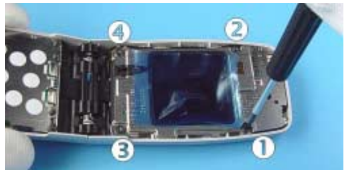
10.) Unscrew the four Torx Plus ® size 6 screws of Upper Block. For assembly, the reverse order and a Torx Plus ® driver with a torque of 27Ncm has to be used.
