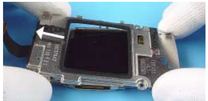
31.) Separate the C2-Cover from LCD CAN Assy.
