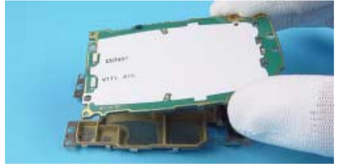
37.) The Engine Module can be removed easily.
