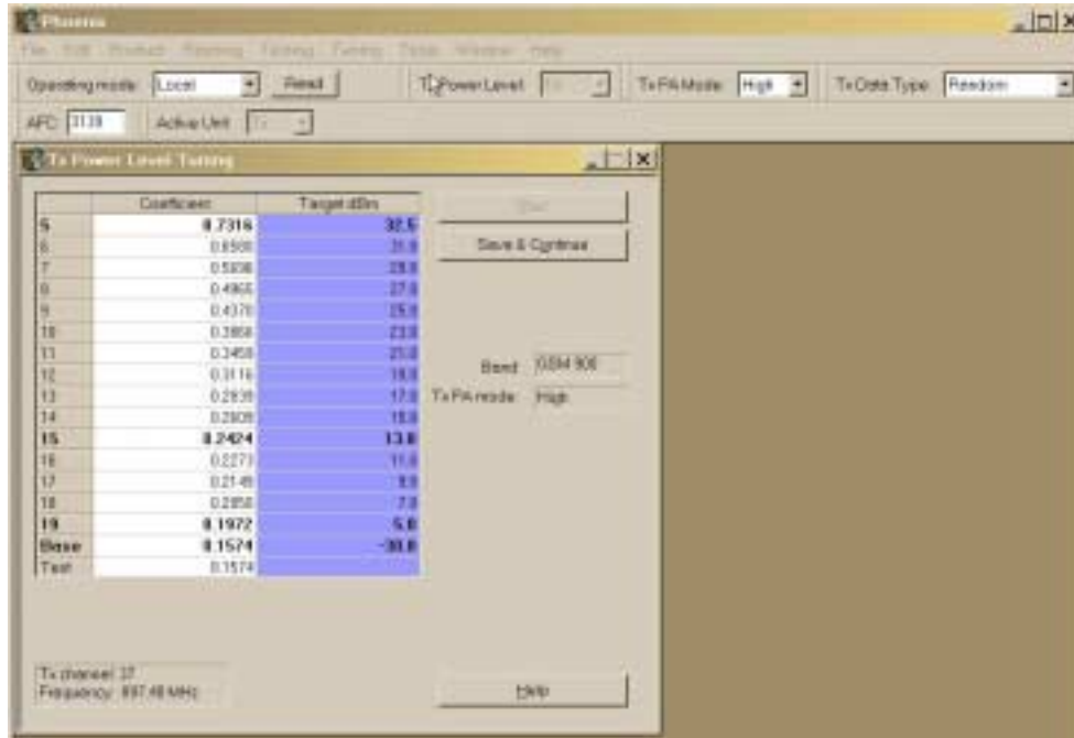
Figure 11: TX Power Level Tuning values for GSM1800 (and GSM1900)
