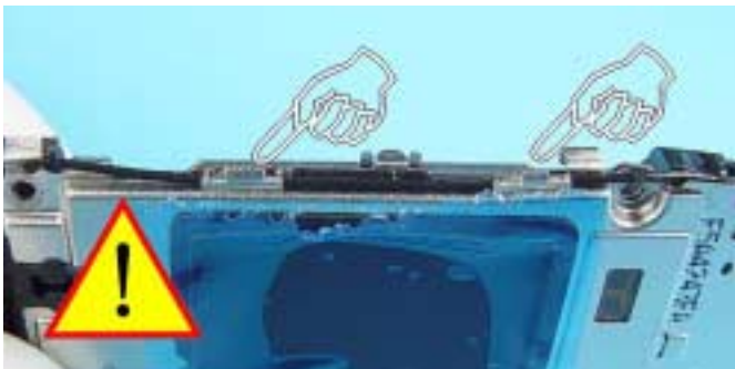
16.) Placement of the Coax Cable in the Upper Block.
