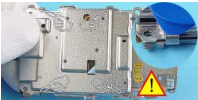
30.) Release the four hooks carefully by using the SRT-6.
