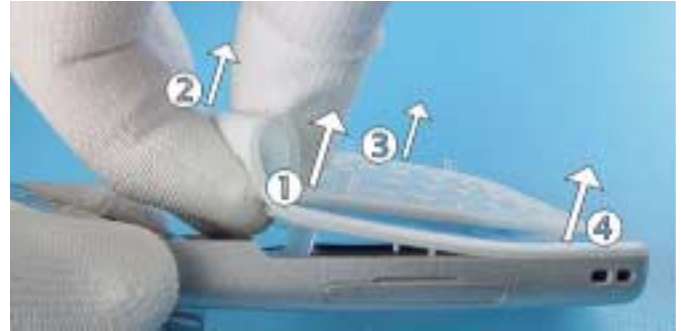
8.) Remove the A-Face Assy from the B-Cover Upper Block carefully.
