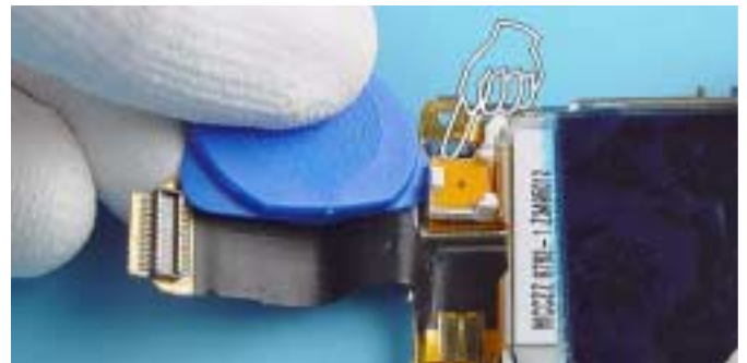
33.) Open the LCD Connector by using the SRT-6 carefully.
