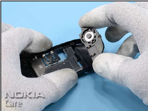
13. ...and remove it from the D-COVER.
