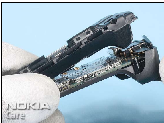
7. Separate the D-COVER from the C-COVER.
