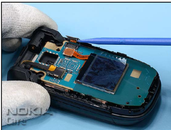
10. Gently open the connector of the LCD PM 128x160 with the SS-93.
