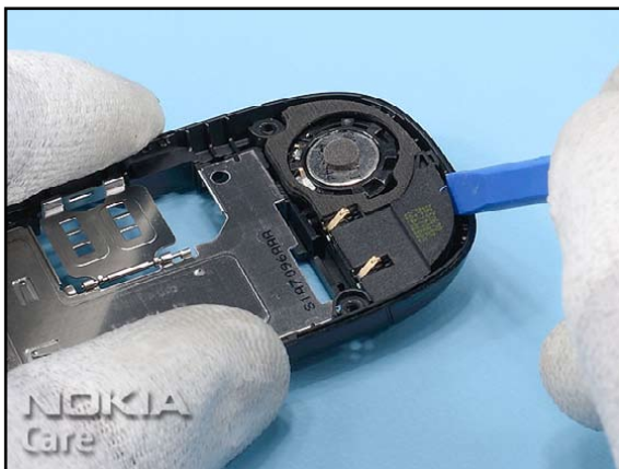
12. Unlock the ANTENNA MODULE with SS-93...
