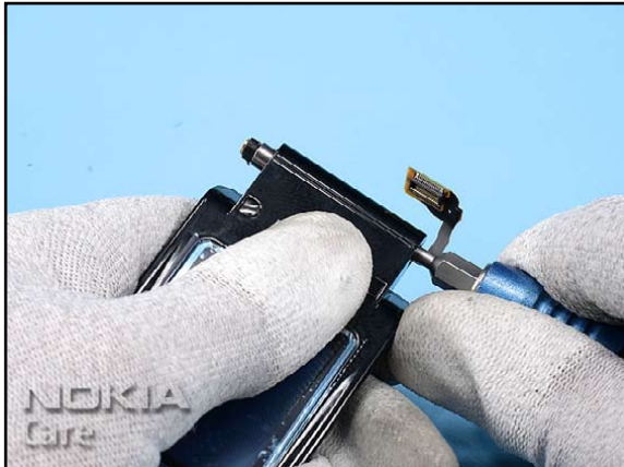
22. Push out the HINGE MODULE from the B-COVER...
