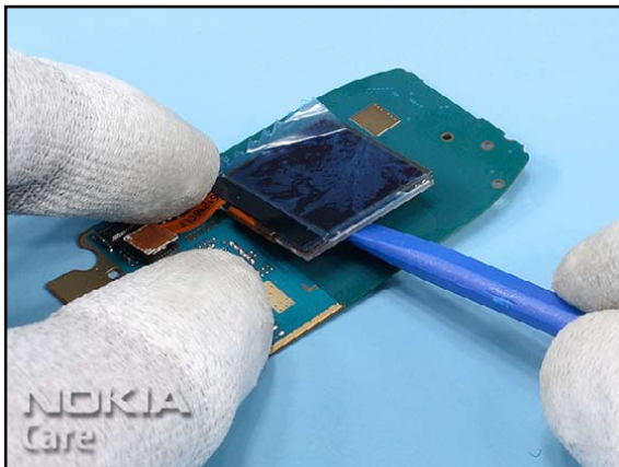
16. Carefully separate the LCD PM 96x68 from the UI PWB ASSY.
