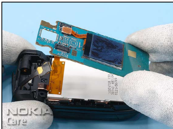
13. Remove the UI PWB ASSY from the B-COVER.
