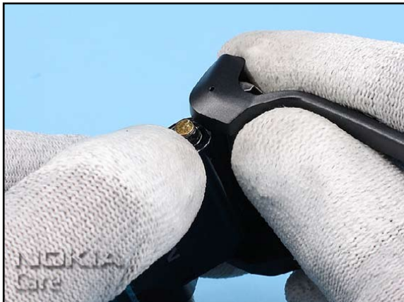
16. Gently open the Hinge but do not separate the parts yet.
