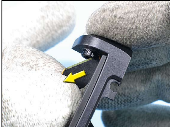
20. Turn around the Upper Block and the C-COVER and remove the end of the PWB FLEX (FPC B2B ASSY).
