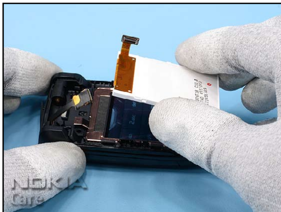
14. Remove the LCD PM 128X160.
