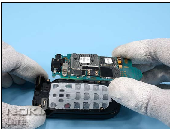
10. Remove the ENGINE MODULE.
