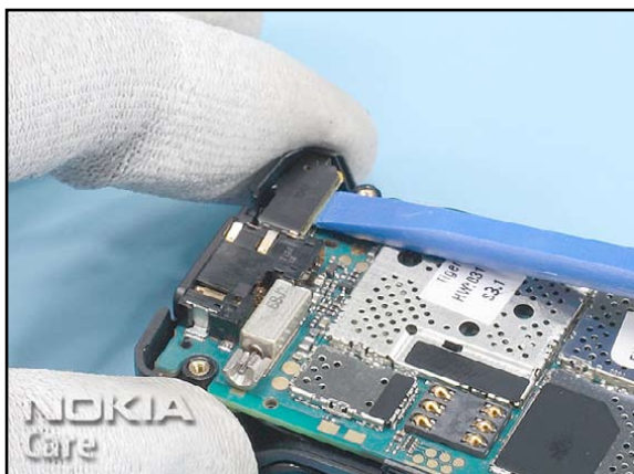
9. Gently open the PWB FLEX connector with the SS-93. Avoid damaging surrounding components.
