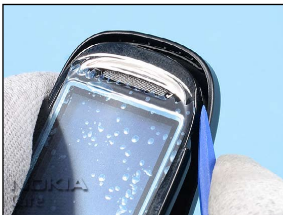
8. Carefully unlock the A-COVER on the top.
