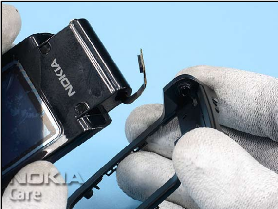
21. Now, separate the C-COVER from the Upper Block.
