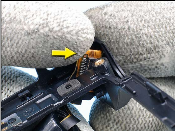
19. Press the end of the PWB FLEX (FPC B2B ASSY) into the direction shown.
