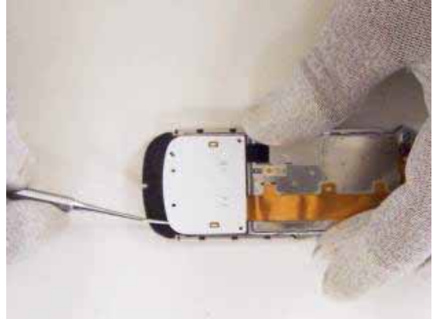
22) Use the dental pick to release the UI Flex.
