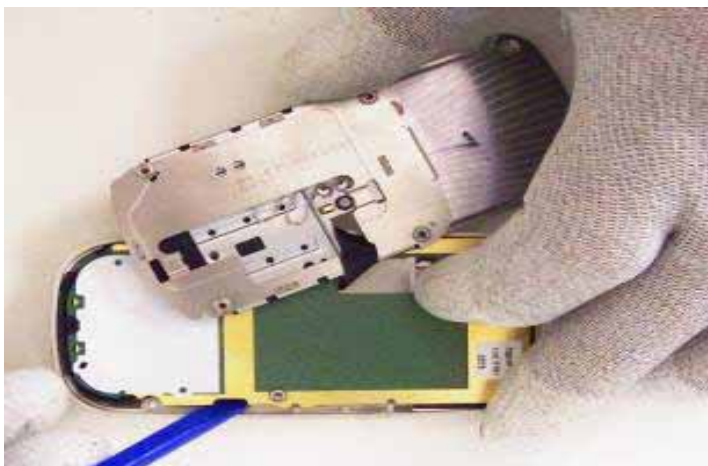
19) Hold the slide module and insert the SS-93 tool to release the D-Cover tabs.
