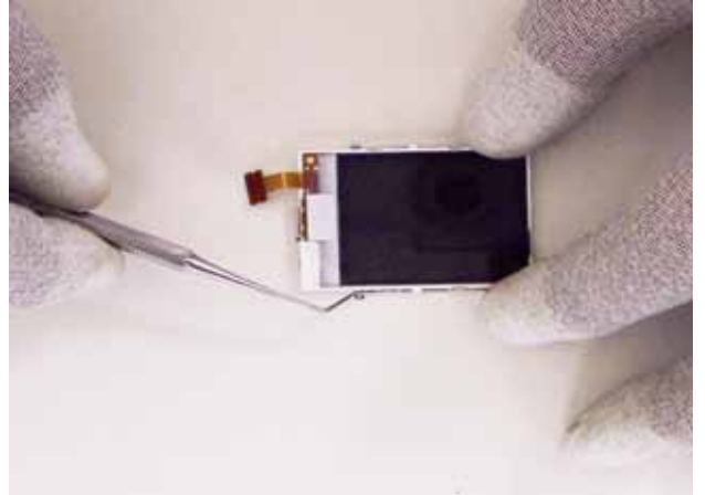
16) Use the dental pick to release the tabs on both sides of the LCD support.
