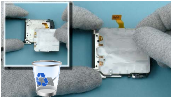
27) Remove the UI FLEX assy. The UI flex cannot be used again. Discard it.
