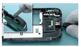
22) Release the DC jack with the charger plug by lifting up the DC jack. Then remove the DC jack. Remove also the USB door.
