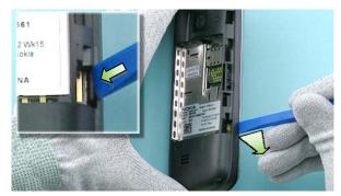
6) Place the SS-93 between the A-COVER ASSY and D-COVER ASSY. Detach the clips by sliding the SS-93 between the covers.
