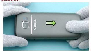
3) To remove the B-COVER ASSY, press and push it in to the direction shown.
