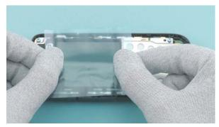
9) Protect the LCD with protective film.
