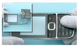
8) Separate the KEYMAT ASSY from the A-COVER by pressing the keymat lightly. When the keymat is separated protect both sides of the window with protective film to avoid scratches.
