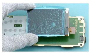
16) Remove the LCD AM TFT.
