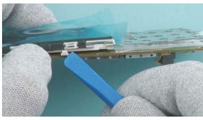
13) Nokia 2730: Separate the UI SHIELDING ASSY by detaching the hooks on both sides with the SS-93 tool.
