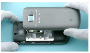
4) Remove the B-COVER ASSY. If there is a battery inserted, remove it also.
