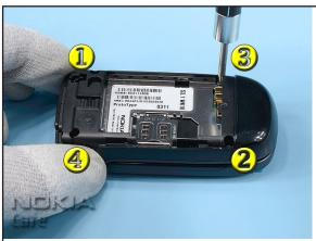
6. Tighten the four screws to the torque of 15Ncm in the order shown.
