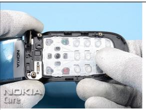
4. Fit the KEYMAT before starting the assembly procedure.
