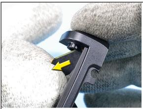
20. Turn around the Upper Block and the C-COVER and remove the end of the PWB FLEX (FPC B2B ASSY).
