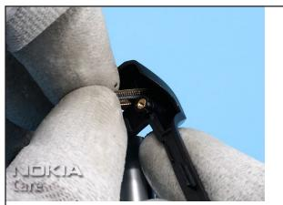
17. Carefully move the PWB FLEX into the hole of the C-COVER... 18. ... as shown in the picture.
