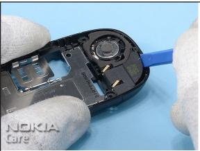
12. Unlock the ANTENNA MODULE with SS-93...
