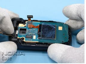
2. Place the UI PWB ASSY onto the B-COVER paying attention to the guide pins of the B-COVER.
