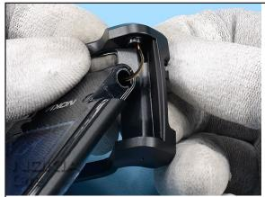
1. Very gently, put the PWB FLEX into the slot of the C-COVER. Avoid squeezing the flex.
