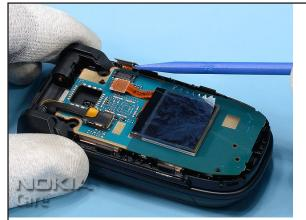
11. Gently open the connector of the LCD PM 128x160 with the SS-93.
