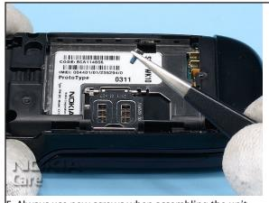
5. Always use new screws when assembling the unit.
