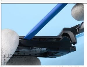
6. Also open the snaps on the left and right side of the Lower Block.
