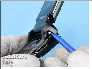
5. Open the Lower Block with the SS-93 starting on the hinge side.
