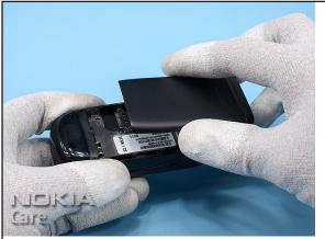
3. Unlock and remove the BATTERY COVER. Remove the battery if inserted.
