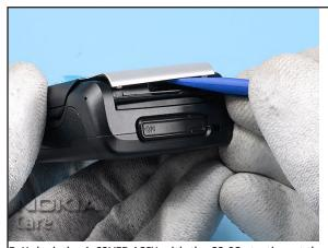
5. Unlock the A-COVER ASSY with the SS-93 starting at the hinge side.
