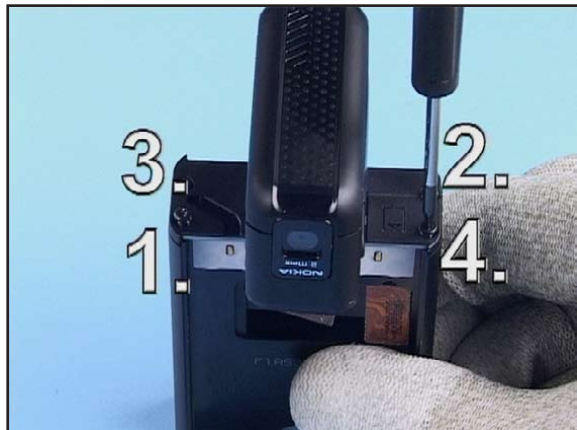
22. Unscrew the 4 screws in the order shown.
