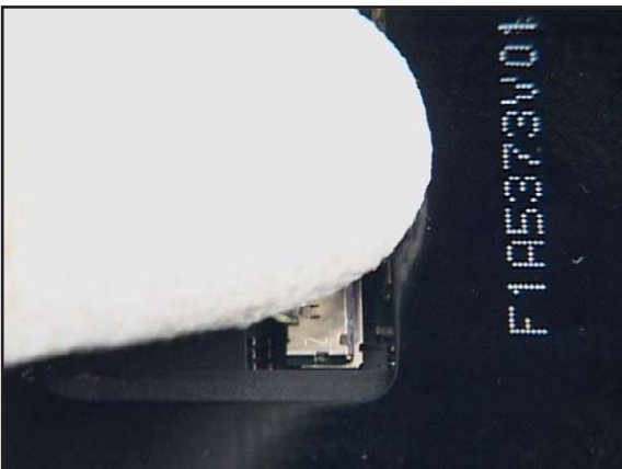
17. Close the UPPER BLOCK CONNECTOR by using finger pressure.
