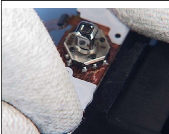
5. Now fix the MAIN FLEX ASSEMBLY to the UPPER FRAME ALUMINIUM using finder pressure.
