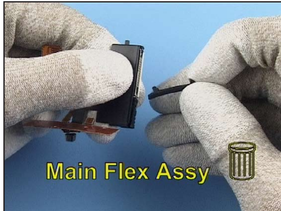
28. The POP PORT DOOR can be pulled out easily. Always use a new MAIN FLEX ASSEMBLY when reassembling.
