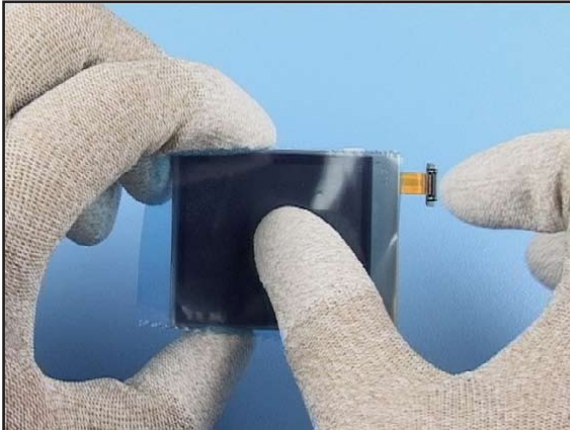
13. Cover the display with a protective film.
