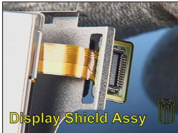
12. Carefully slot through the flex connector. Always use a new DISPLAY SHIELD ASSEMBLY when reassembling.
