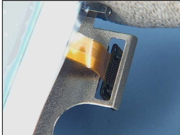
20. Slot through the flex foil of the LCD MODULE.
