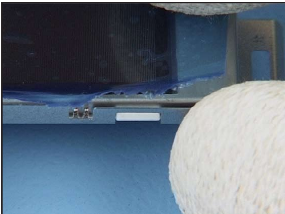
21. Fix all metal latches of the DISPLAY SHIELD ASSY.
