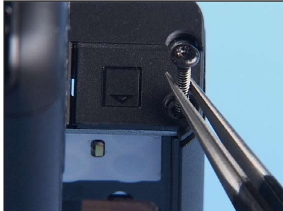
8. Insert the screws with tweezers, note the different screw types.
