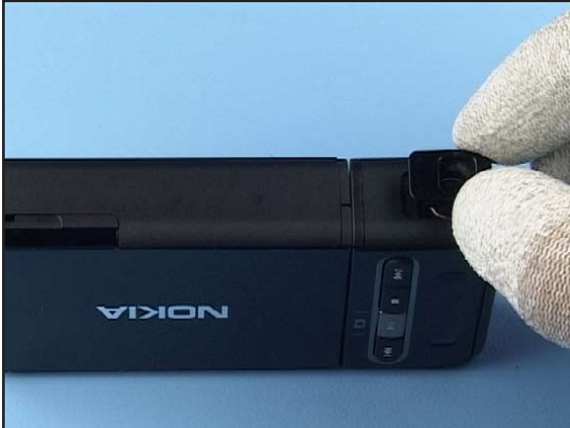
25. Place the CAMERA LENS ASSEMBLY and fix it.
