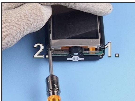
27. Tighten the screws in the order shown, using a torque of 18 Ncm.
