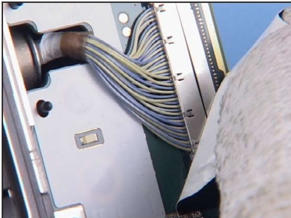
9. Peel up the COAX CABLE SUPPORT TAPE
