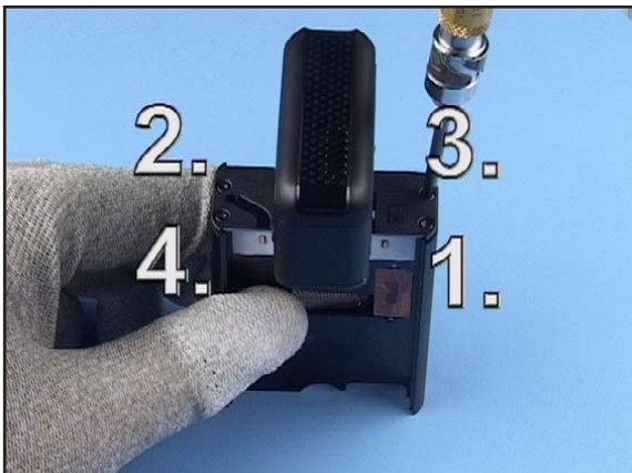
11. Now, tighten the screws with the correct torque in the order shown, using a torque of 18 Ncm .
