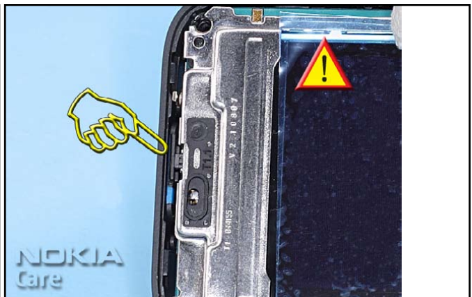
6. Take special care to the power switch when assembling the unit.
