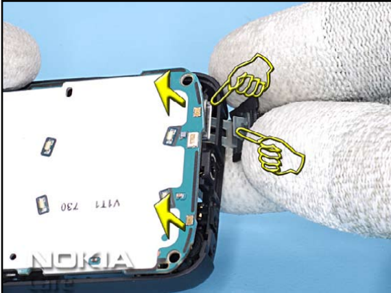
7. Lift a bit the PWB and fit the USB DOOR into its place. Check its correct position.
