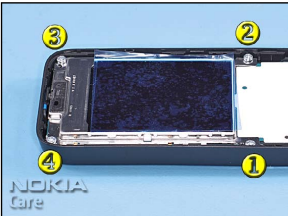
9. Tighten the screws with a torque of 20Ncm in the order shown.
