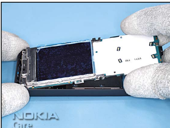
5. Place the PWB into the B-COVER ASSY as shown.
