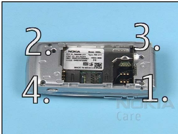
14. Tighten the 4 screws in the order shown.
