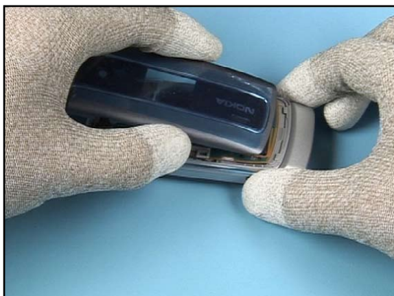
31. Now place the A-COVER, beginning with the top clips.
