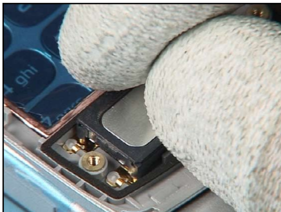
14. Mind the correct polarity of the terminals. Slightly push it into its place.
