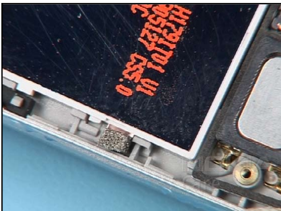
17. Note the grounding pads on both sides of the display before going on.
