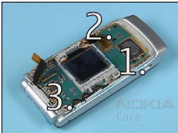
13. Unscrew these 3 screws in the order shown. Discard these screws. Do not use them again.
