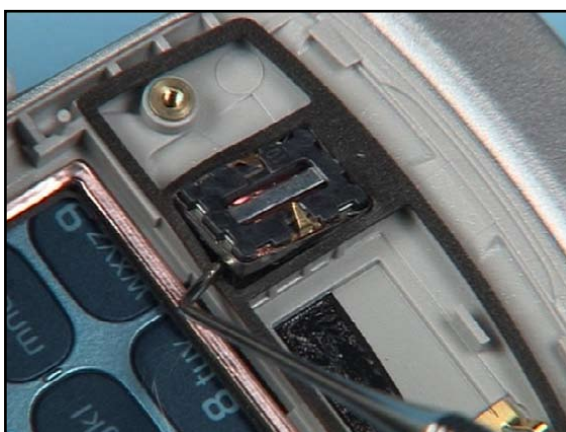
22. Ease out and remove the EARPIECE with the dental pick.
