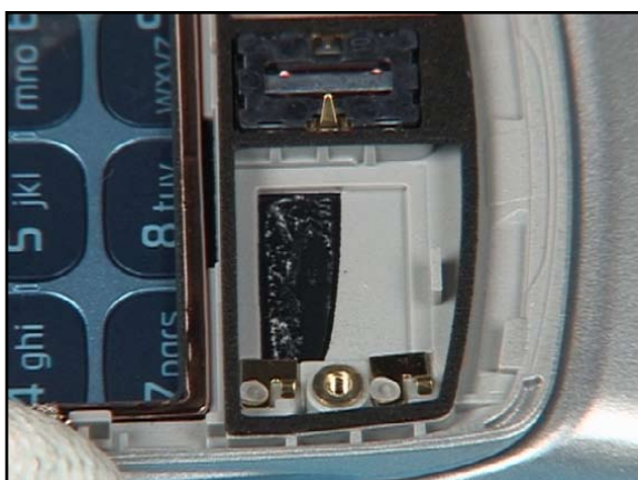
21. Remove the adhesive residues of the IHF SPEAKER ADHESIVE completely if the cover should be used for reassembling again.
