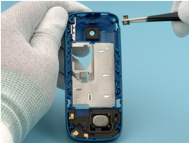
19. Remove the charge jack with tweezers.
