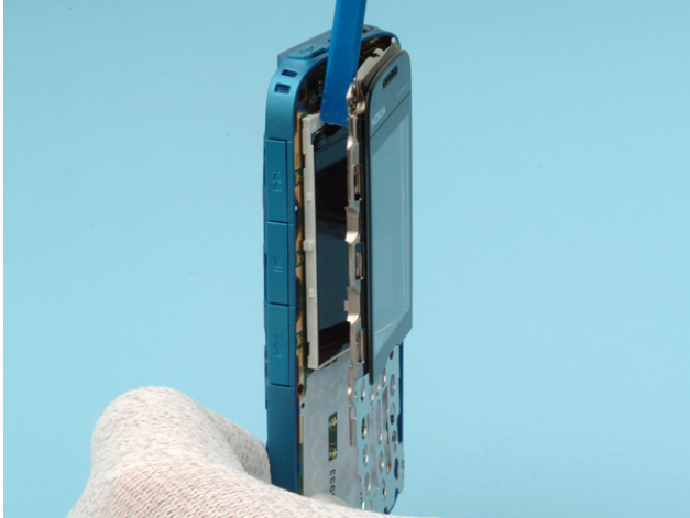
13. Release the clips holding the UI shield. Use the SS-93 tool and start on any side.
