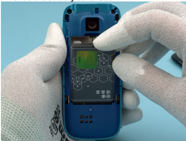
3. Lift and remove the battery.
