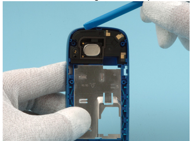
20. Remove the camera gasket as one piece.
