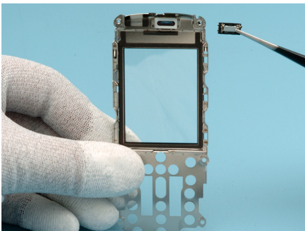
35. Remove the earpiece speaker with tweezers. End of disassembly.
