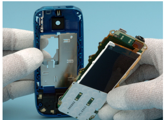
16. Remove the engine module.
