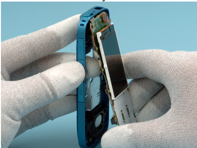
15. Lift and pull back slightly the engine module to free the USB connector.
