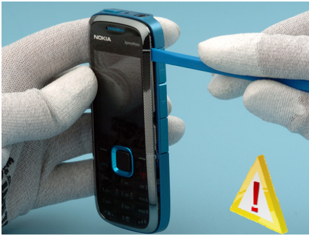
7. Carefully wedge the SS-93 tool under the edge of the A-cover and work carefully around the A-cover.
