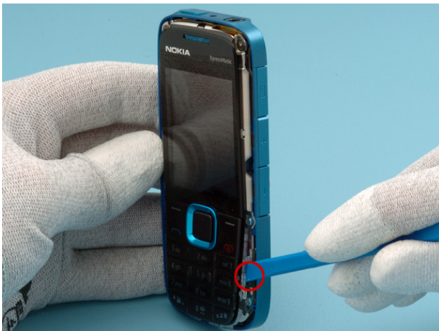
9. Release the clips on both sides of the keymat. Use the SS-93 tool and insert it from the right side first.
