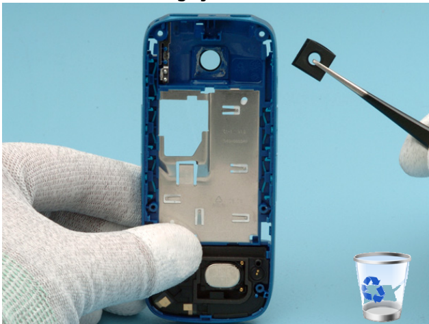
19. Remove the charge jack with tweezers.
