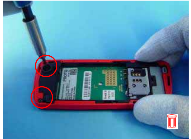
2) Use T5+ to remove the screws.
