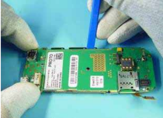
11) Detach the UI SHIELD ASSY from PWB.
