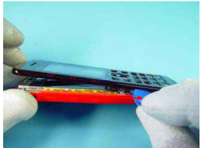
3) Detach the snaps of A-COVER ASSY with SRT-6 by sliding from top to bottom side. Do the same on the opposite side.
