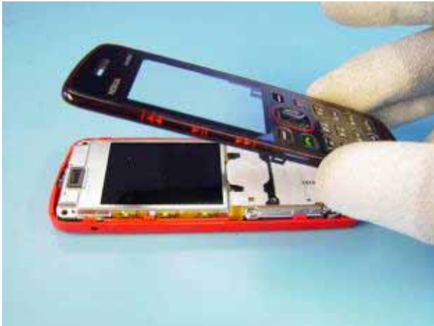
4) Remove the A-COVER ASSY inclusive KEYMAT.
