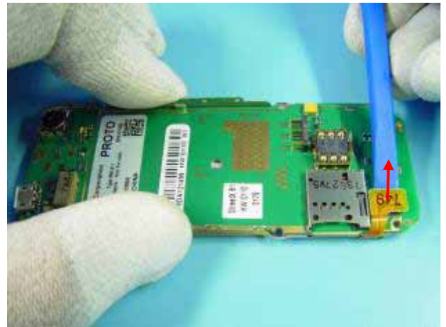
10) Disconnect the UI SHIELD ASSY with SS-93.
