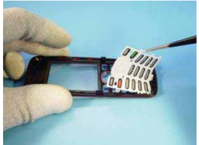
5) KEYMAT can be taken away with tweezers.
