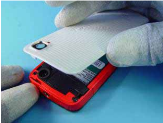
1) Press the battery release button to remove the C-COVER ASSY.
