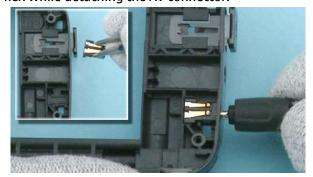
24) Use the charger plug to detach the DC jack from C-COVER ASSY. Remove the DC jack with the tweezers.
