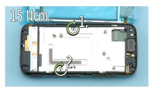
5) Tighten the two TORX + size 4 screws to the torque of 15 Ncm in the order shown.
