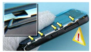
8) Use the dental tool to carefully release the clips holding the TOUCH WINDOW ASSEMBLY.
