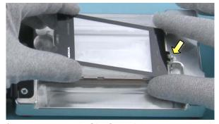
2) Remove potective film from the TOUCH WINDOW ASSEMBLY before placing the assembly. Use the guiding on bottom side to position the assembly correctly.
