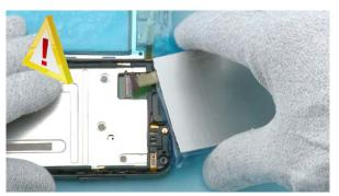
12) Carefully disconnect the LCD connector and remove the LCD.
