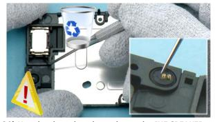
30) Use the dental tool to release the IHF SPEAKER. Be careful not to damage the IHF gasket! The speaker and the speaker adhesive cannot be reused. Also remove the MICROPHONE with the dental tool.
