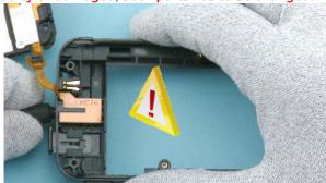
22) Push out the audio connector with the AV plug. Be careful not to damage the audio connector while releasing it - or the flex soldering! Avoid pulling the flex while detaching the AV connector!
