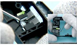
28) Push the end of the USB DOOR with the dental tool as shown.
