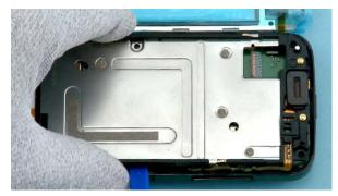
15) Use the SS-93 to carefully lift up the UI DECK to gain access to the upper flex connector.
