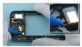
25) Use the sharp end of the SS-93 to release the clip holding the ANTENNA ASSEMBLY.
