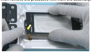
3) Then place the top side of the TOUCH WINDOW ASSEMBLY using the guide of the SS-214.
