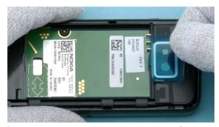
4) Protect the camera lens with protective film.
