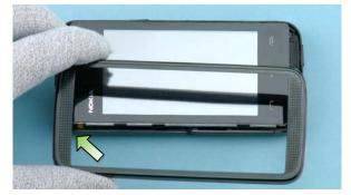
6) Remove the A-COVER. Make sure the speaker mesh stays in its place underneath the cover .
