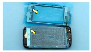
10) Protect the inner side of the TOUCH WINDOW ASSEMBLY and the LCD with protective film.
