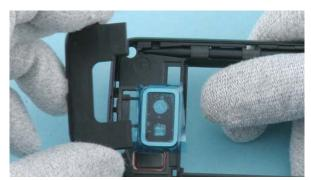
26) Turn the C-COVER over and detach the ANTENNA ASSEMBLY.
