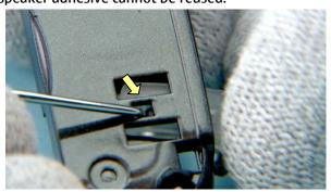
29) Turn the C-cover over. Push the clip with the dental tool and keep the clip pressed while pulling the door out.
