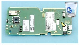
34) Remove also the LNA SHIELD LID from the bottom side of the engine board.
