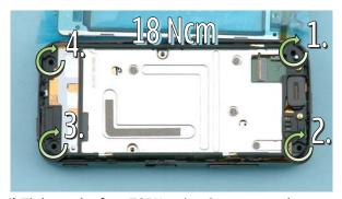
4) Tighten the four TORX + size 6 screws to the torque of 18 Ncm in the order shown.
