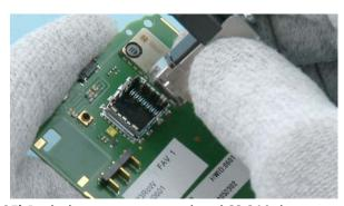
35) Push the camera removal tool SS-210 down until the camera retaining clips are released. Lift up the SS-210 - and remove the CAMERA.
