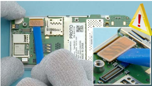
15) Open the UI FLEX connector with the SS-93. Be careful not to damage the connector or the components nearby!
