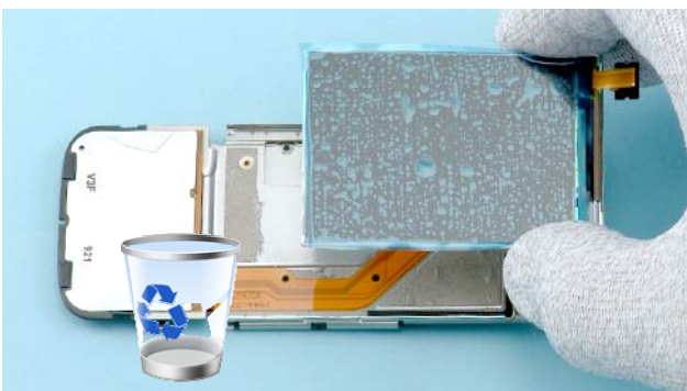
29) Remove the LCD. The LCD cannot be used again. Discard it.
