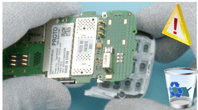
18) The NUMERIC KEYPAD is glued to the engine board. While removing the keypad be careful not to damage the components on the engine board! The NUMERIC KEYPAD has always to be renewed.
