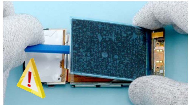
28) Carefully push the SS-93 under the LCD to detach the LCD completely. Lift up the LCD as shown. Be careful not to damage the UI FLEX underneath the LCD!
