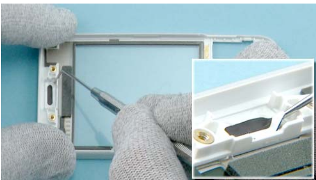
33) Use the dental tool to release the EARPIECE ADHESIVE.
