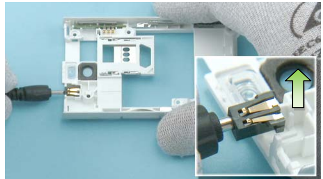
10) Use a DC plug to lift up the DC JACK.
