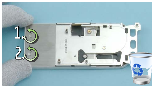
20) Unscrew the two TORX + size 4 screws in the order shown. Do not use them again.
