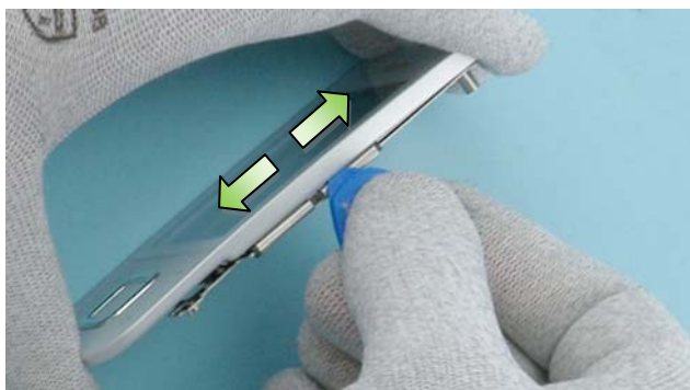
23) Release also the clips on the other side of the device.
