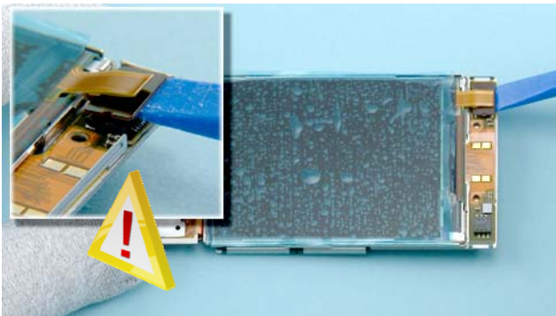
25) Use the SS-93 to open the LCD connector. Be careful not to damage the connector!
