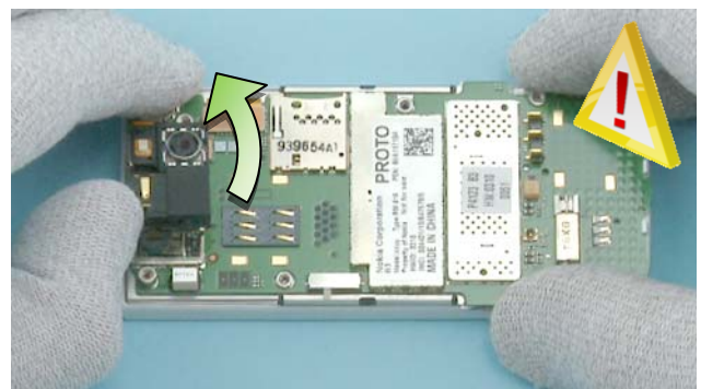
12) Carefully turn over the DOCKING FLEX MODULE to gain access to the connector underneath.
