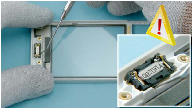
31) Use the dental tool to lift up the EARPIECE. Be aware of the sharp point of the dental tool - be careful not to injure yourself.
