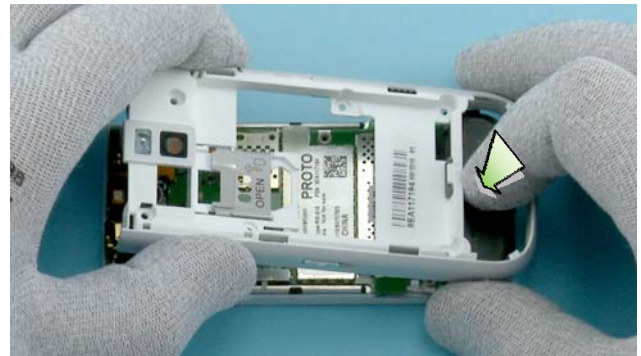
8) Push the ANTENNA MODULE ASSY slightly towards the engine board and detach the D-COVER ASSY.
