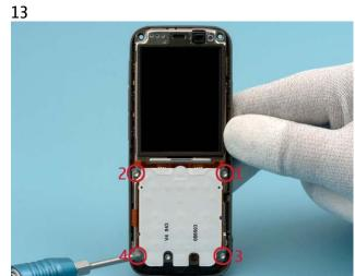
Unscrew the four T6+ screws.
