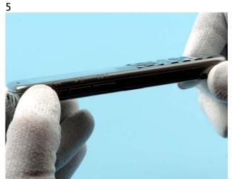
Check that the A-COVER has been closed properly before you tighten the screws.
