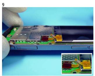
This is the position of the LCD FLEX after the prebending procedure. Make sure the connector is secure by pressing it.
