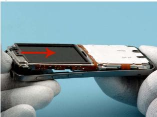
To remove the assembly, stretch the C-COVER outwards over the audio connector.
