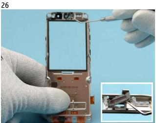
Use the dental tool to lift and release the adhesive net.
