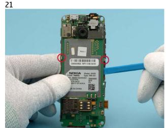
Release the clips on both sides of the PWB.
