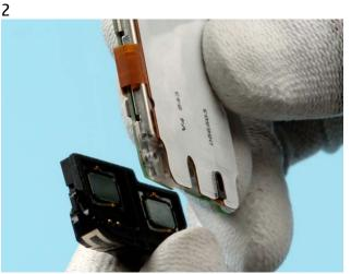
Place the ANTENNA MODULE and PWB against each other.
