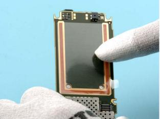
Make sure that the LCD ADHESIVE is glued to the PWB.
