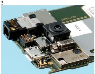
This is the position of the CAMERA and CAMERA BOOT in place.
