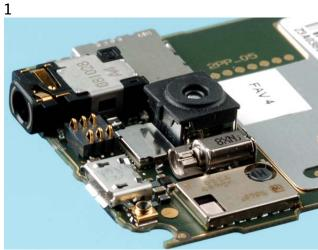
When assembling the C-COVER, check that the CAMERA BOOT is in the correct position.
