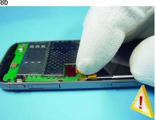
Do not press the LCD FLEX down too hard because it can cause sharp curves and break it.
