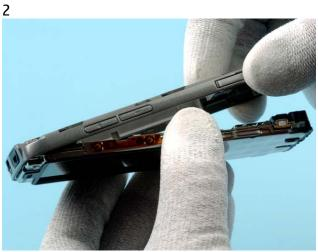
Start assembling the C-COVER from the audio connector.
