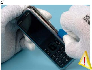
Carefully wedge the SRT-6 tool under the edge of the A-COVER and work carefully around the cover to release the 7 clips. **Note**: Be careful with the clips, they break easily.
