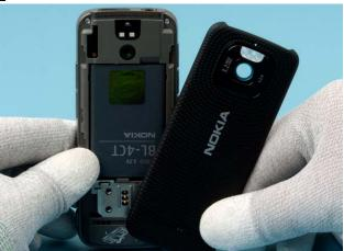
Remove the BATTERY COVER and remove the battery.
