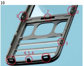
Before removing the A-COVER, make sure that you have released all 7 clips.
