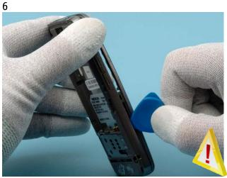
Pull the C-COVER outwards around the cover with the SRT-6 tool when opening the A-COVER.
