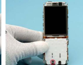
Unscrew the T6+ screw to remove the antenna.
