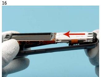
Stretch the C-cover outwards to release the clip which holds the assembly in place.
