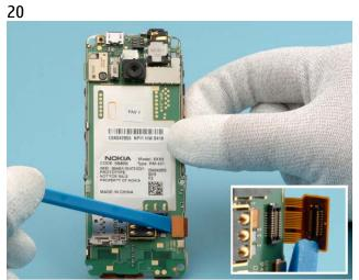
Use the SS-93 tool to release the connector of the UI.
