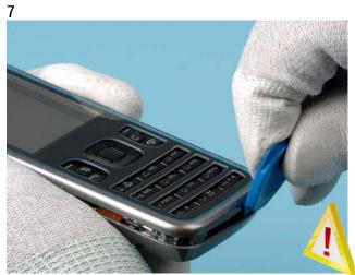
Pull the C-COVER outwards to carefully release the lower side clips.
