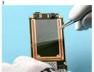
Remove the protective foil with tweezers.
