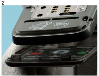
First assemble the lower clips of the A-COVER.
