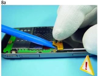
Carefully press the LCD FLEX down.
