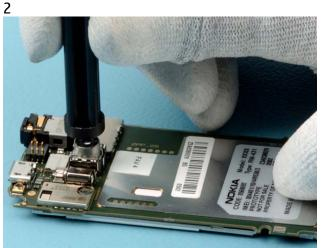
Turn the camera removal tool upside down and use its other end to push the CAMERA until you hear a "click" sound.
