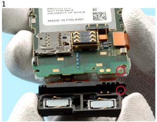
Use the guiding pin in the ANTENNA MODULE and the hole in the PWB when assembling the ANTENNA MODULE.
