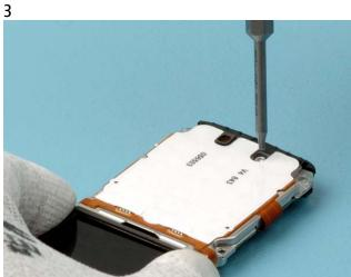
Tighten the screw to the torque of 13 Ncm.
