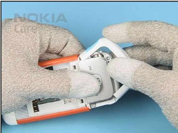
19. Fit the BOTTOM COVER ASSY.
