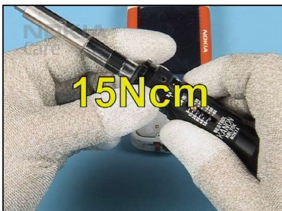
11. Set the torque driver to the correct torque...
