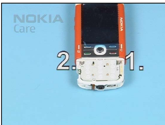
12. Tighten the screws in the order shown, starting on the D-COVER NUMERIC side.
