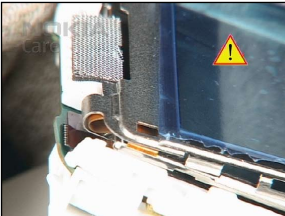
21. Gently fit the FRAME LCD ASSY. Take care to the LCD flex...
