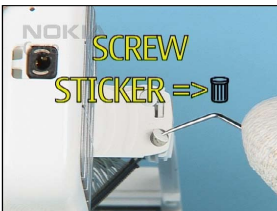
36. Turn the LOWER BLOCK to the shown position. Remove all SCREW STICKERS and discard them.
