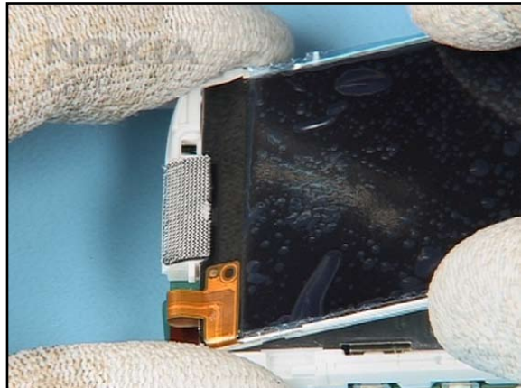
20. Place the LCD into the FRAME UPPER ASSY, starting on the shown side.
