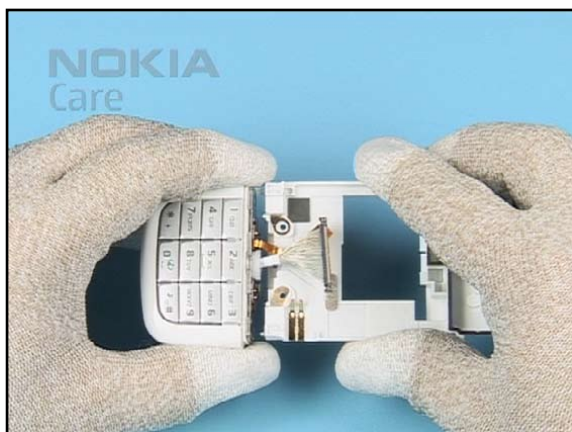
39. Separate the C-COVER ASSY from the LOWER BLOCK.
