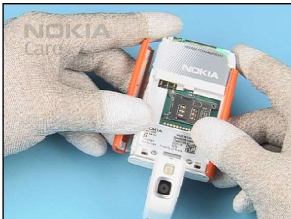
9. Remove the SIDE ASSY RIGHT.
