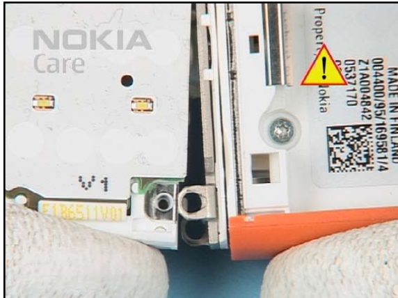
14. Gently separate the Lower Block from the Upper Block, starting at the shown side.
