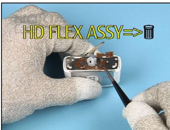
40. Remove the HD FLEX ASSY and discard it.
