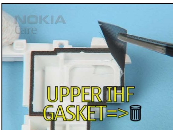
35. Remove the UPPER IHF GASKET and the adhesive residues.
