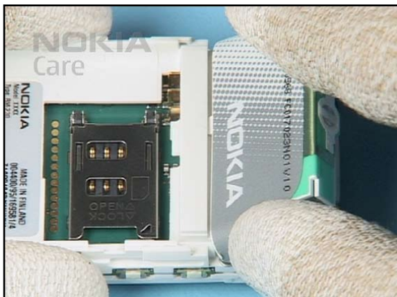
25. Insert the ANTENNA ASSY, paying attention to the guide pin. Secure the ANTENNA ASSY by pressing it into place.
