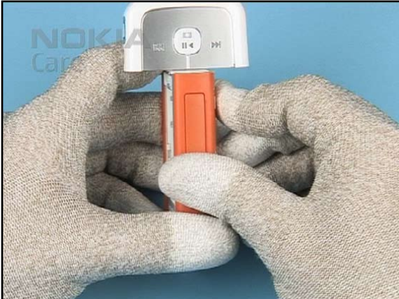
31. ...and slide the SIDE ASSY RIGHT into its place.
