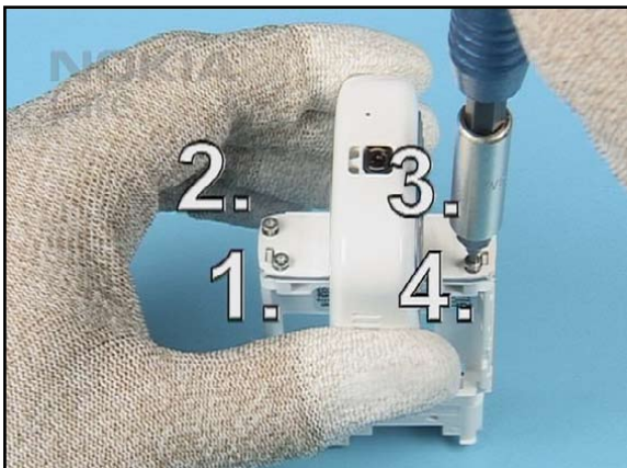
37. Undo the screw in the order shown.
