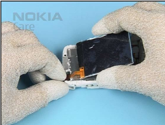
19. Close the LCD connector.
