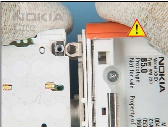
15. Now, separate the other HINGE side. Take care to the COAX CABLE.
