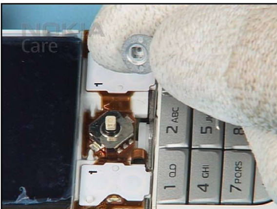
23. Fit the JOYSTICK COVER. Note its correct position.
