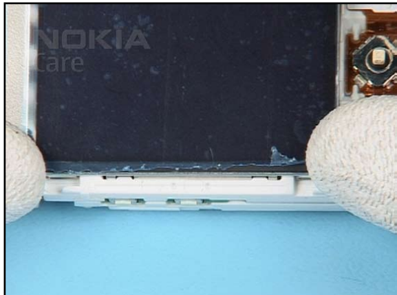
22. ...and secure the FRAME LCD into its place.
