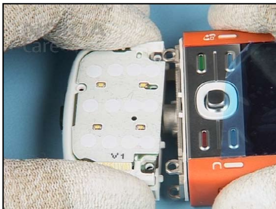
8. Fit the D-COVER NUMERIC ASSY.
