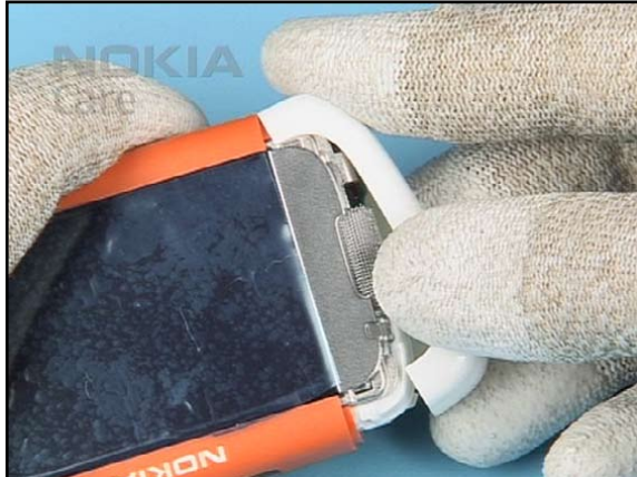
32. Fit the TOP COVER at the shown side first...
