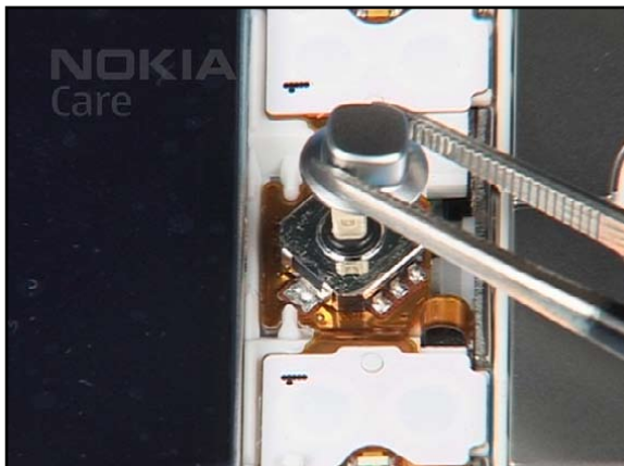
13. Remove the JOYSTICK COVER.
