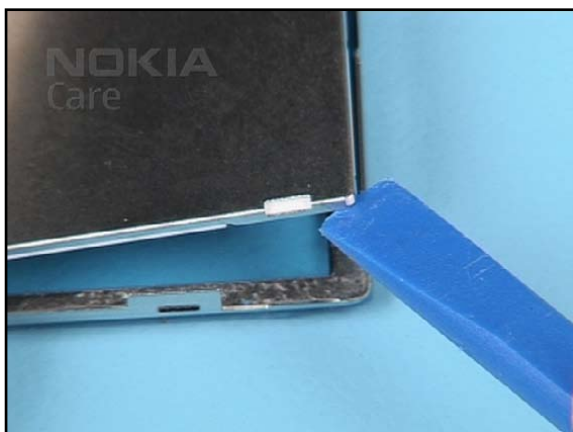
31. Remove the LCD from the FRAME LCD.
