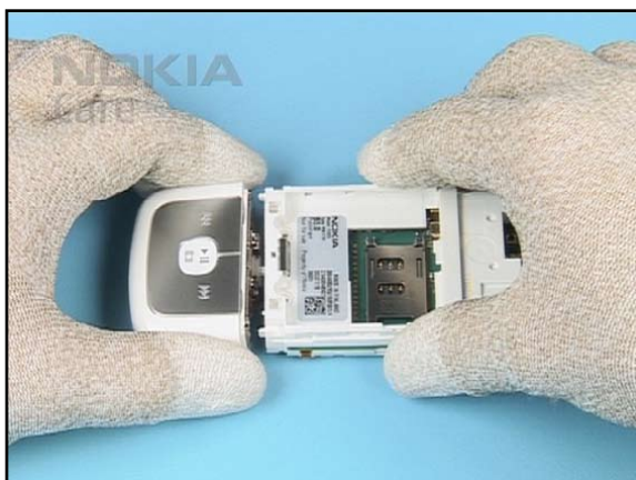
9. Align the HINGE MECHANICAL ASSY with the UPPER BLOCK...
