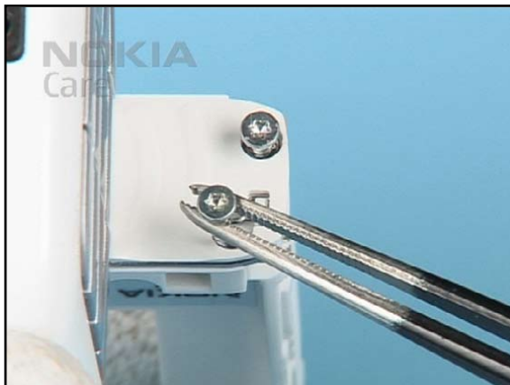
38. Remove the screws.
