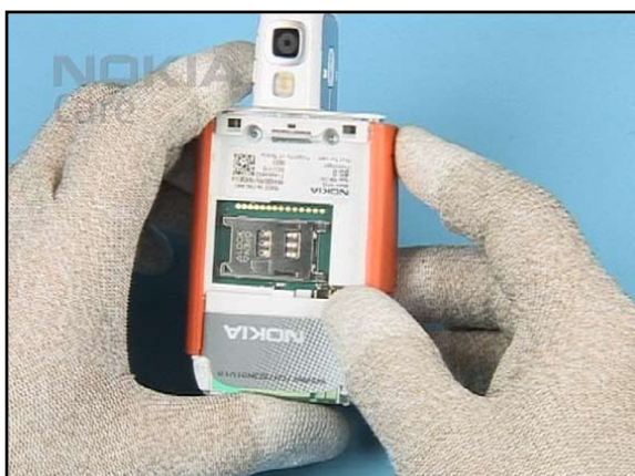
29. Align the SIDE ASSY RIGHT with the UPPER BLOCK.
