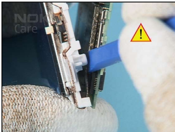
26. First open the FLEX UPPER connector...
