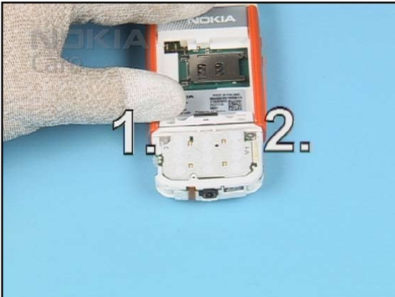
13. Undo the last two screws in the order shown and remove them, too.
