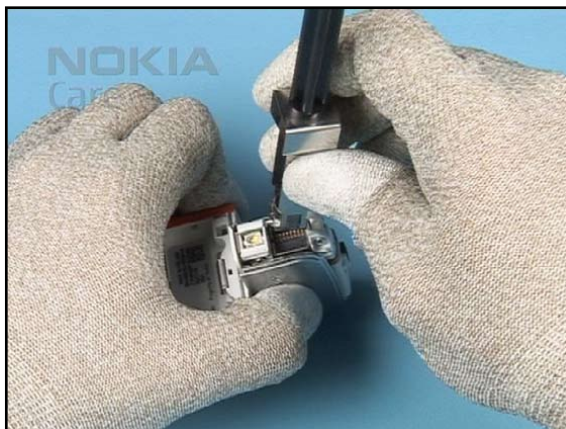
8. Unlock and remove the CAMERA with the SS-45.
