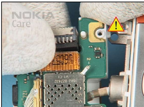
7. Place the LOWER FLEX ASSY with the CAMERA housing into its place and close the connector.
