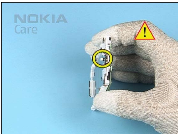
3. Take special care to the JOYSTICK during assembly.
