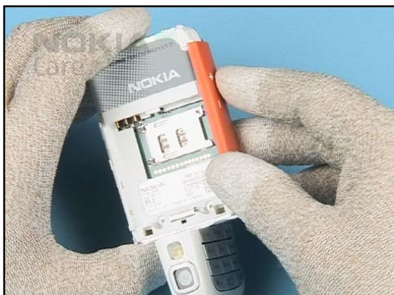
27. Align the SIDE ASSY LEFT with the UPPER BLOCK.
