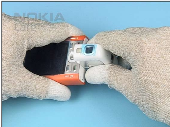
20. Finally, check the mechanical functionality of the HINGE and that no gaps remain.
