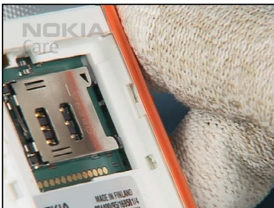
28. Check the correct position of the guide pins. Slide the SIDE ASSY LEFT into its place.
