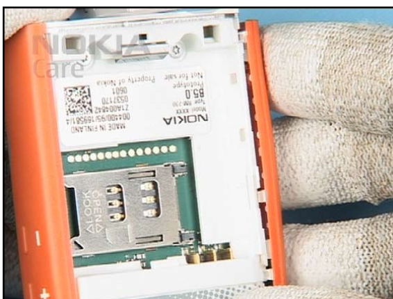
30. Check the correct position of the guide pins...
