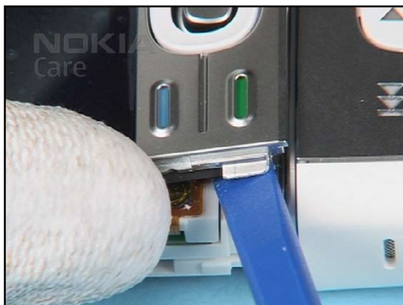
12. Lift the KEYMAT MENU a bit and remove it.
