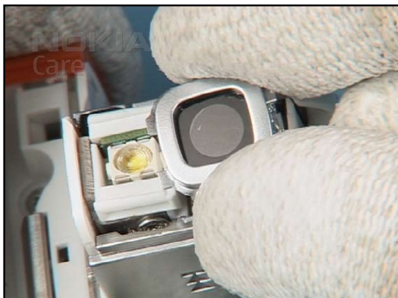
7. Remove the WINDOW CAMERA ASSY.
