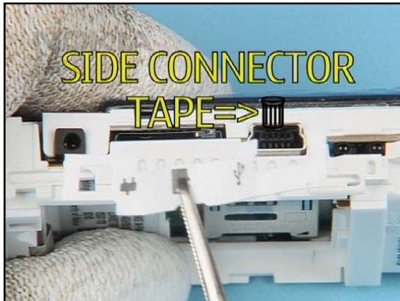
20. remove the SIDE CONNECTOR TAPE and discard it.
