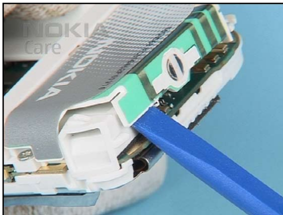
14. Gently unlock the ANTENNA ASSY hooks...
