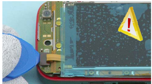
10) Open the LCD connector from the 2 MX UI FLEX ASSEMBLY with the SS-93. Be careful not to damage the connector.
