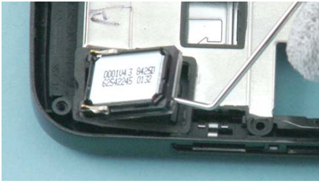
37) Use the dental tool to release the IHF SPEAKER and the IHF SPEAKER gasket.
