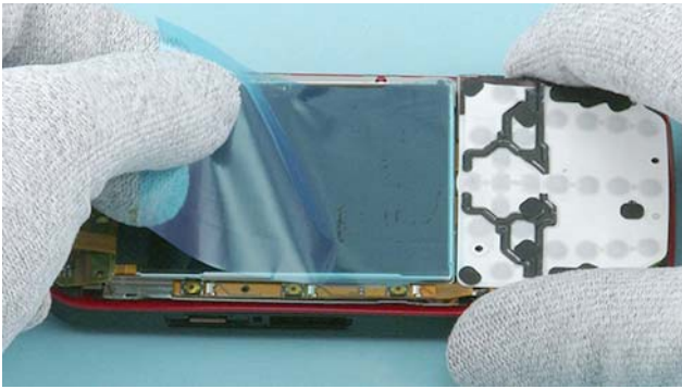
7) Remember to protect the LCD with protective film.
