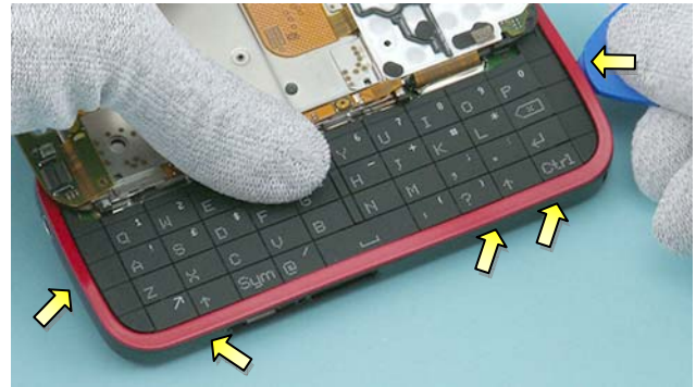
14) Use the SRT-6 to release the clips holding the ACCENT BAND QWERTY.
