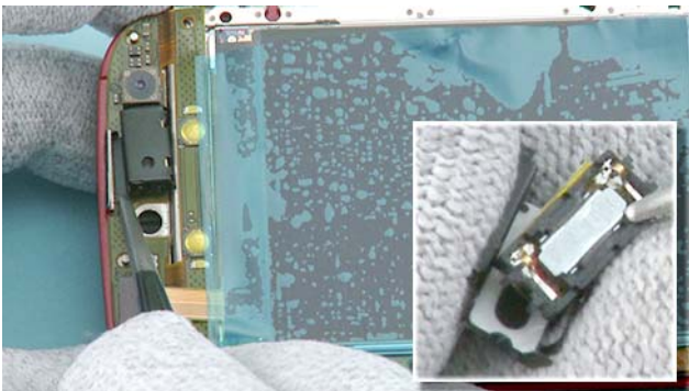
9) Release the EARPIECE HOLDER and remove it with the tweezers. Then separate the EARPIECE from the EARPIECE HOLDER with the tweezers.
