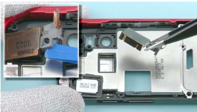
33) Lift up the AV FLEX ASSY with the SS-93 and remove the ASSY with the tweezers.
