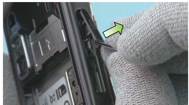
16) Remove the USB-DOOR by pulling it to the direction shown.
