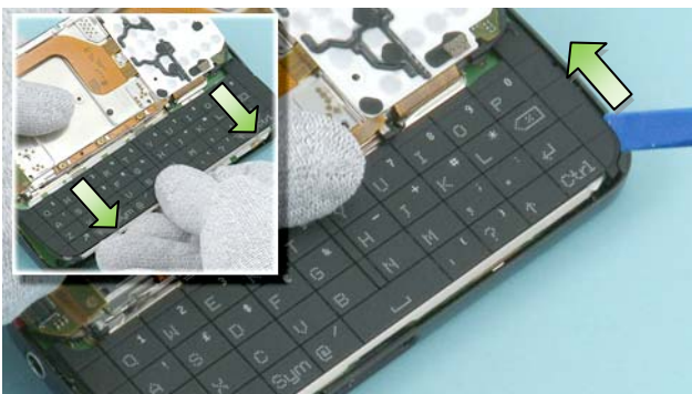
15) Use the SS-93 to detach the QWERTY KEYMAT adhesive on the right side. Pull the QWERTY KEYMAT in the direction shown.
