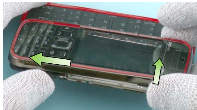
6) Carefully lift up the top side of the A-COVER and at the same time push it to the left so that ITU KEYMAT latches open. Check that ITU latches are not broken.
