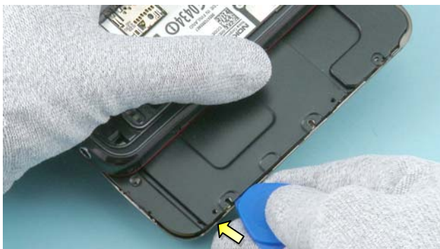
5) Release the A-COVER ASSEMBLY from the SLIDE MODULE using the SRT-6. Carefully open the shown corner.
