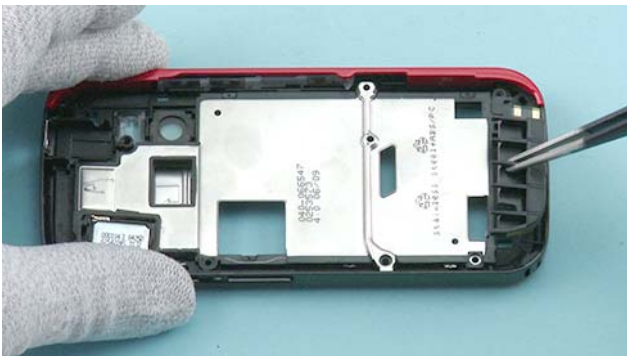
35) Remove the ANTENNA ASSEMBLY with the tweezers.
