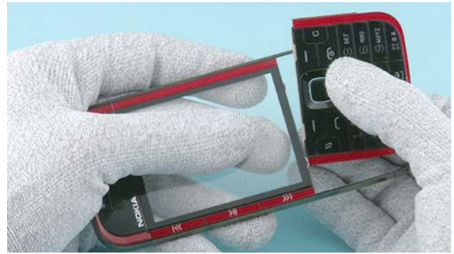
8) Separate the KEYMAT ASSEMBLY from the A-COVER ASSEMBLY.
