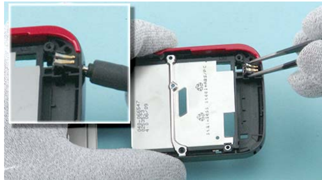
36) Release the DC JACK with the charger and then remove the DC JACK with the tweezers.
