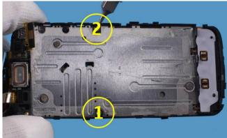
19. Remove the two TORX 5+ screws.
