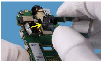
29. Remove CAMERA using SS-102 tool.
