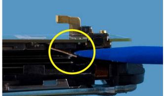
21. Disconnect the **PWB** from the **LCD FRAME ASSY**.
