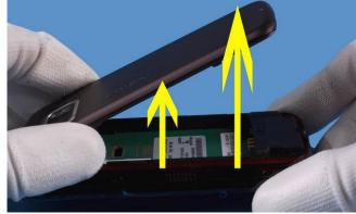
2. Lift up and remove the **BATTERY COVER**.
