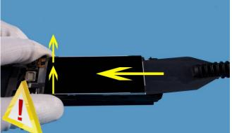
17. Move SS-195 tool underneath the **LCD** in the direction as shown in the picture to lift up the **LCD** on top side of **LCD FRAME ASSY**.
