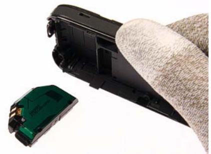
18.) The Antenna IHF Assy drops out when turning the D-Cover Assy .
