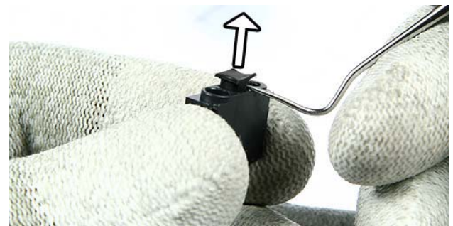
20.) Remove the Easy Flash Connector Cap from the Easy Flash Connector with the Dental Tool .
