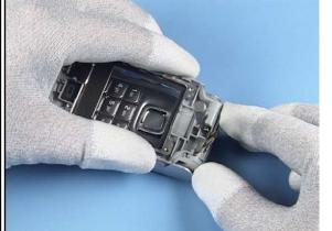
28. Now, the A-COVER UPPER ASSEMBLY can be removed easily. Mind the flex foil. The Hinge can be pulled out after the spring expanding carefully if needed.
