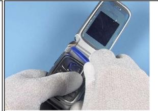
4. Open the assembly, release both upper clips of the ANTENNA CAP.
