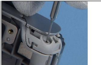
26. Bend down the hinge module with the SS-6 first. Note that the SS-6 is very delicate and can be break easily.
