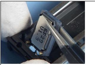
20. Remove it with tweezers now. Bear in mind that the IHF GASKET will be destroyed during the removal and must be renewed when reassembly.
