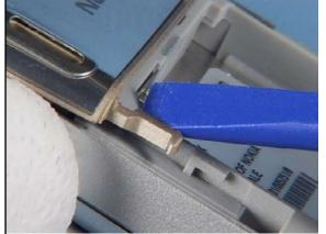
3. Unlock both latches of the ANTENNA CAP.
