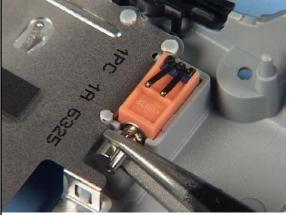
17. Lever out the VIBRA MOTOR.
