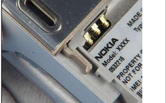
19. Click the snaps into their places, beginning from the upper 20. Note the correct positioning of the snaps gefore going on. side of the ANTENNA CAP.
