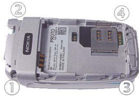
10.) Unscrew the four, Torx Plus® size 6 screws in the shown order. For assembly, use the same order and a Torx Plus® size 6 driver with a torque setting of 17Ncm.
