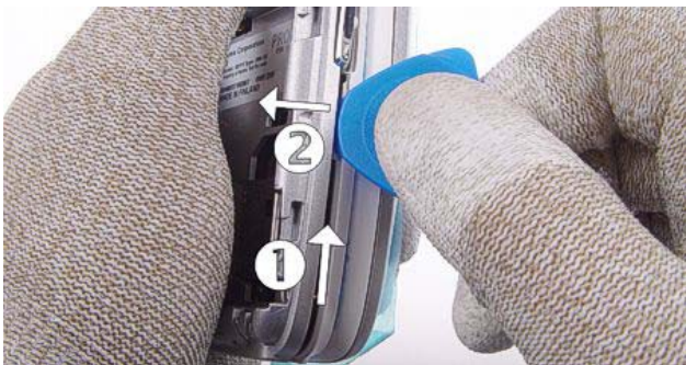
11.) Place the SRT-6 between D-Cover and the C-Cover and shift it carefully along the edge.
