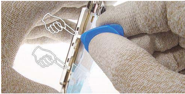
15.) The UI Shield is attached to the UI-Module with four snaps. Release the snaps by using the SRT-6.
