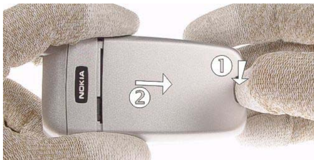
3.) Press the Release Button and remove the E-Cover .
