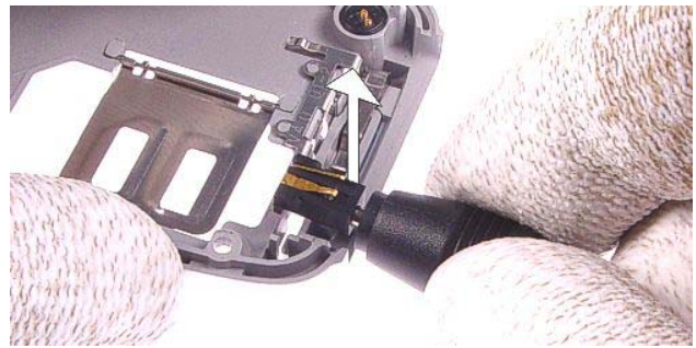
18.) Remove the DC-Jack by using the DC-plug.
