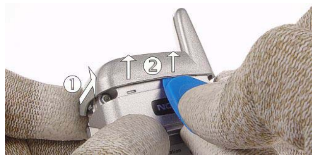
8.) Press the Antenna Cover a bit upward and place the SRT-6 between the Antenna Cover and the D-Cover . Now, pull up the Antenna Cover by releasing the clips.
