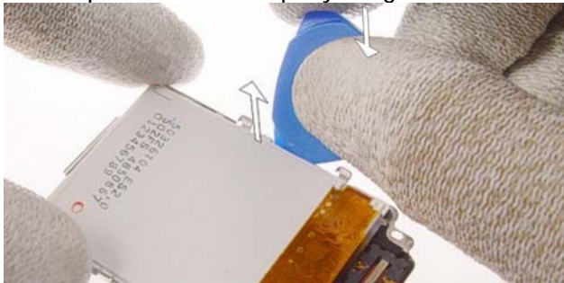
17.) Use the SRT-6 as a lever to remove the LCD Display.
