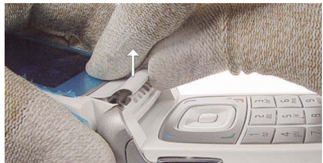
4.) Now, remove the B-Cover Bezel . Use always a new one when re-assembling the unit.
