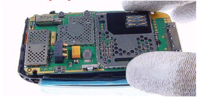
22.) Place the Engine Module on the C-Cover .
