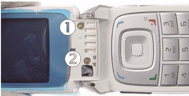
5.) Unscrew the two, Torx Plus® size 6 screws in the shown order. For assembly, use the same order and a Torx Plus® size 6 driver with a torque setting of 17Ncm.
