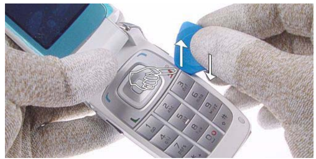
4.) Place the SRT-6 between the Keymat and the edge of the C-Cover and lever out the Keymat as shown in the picture.
