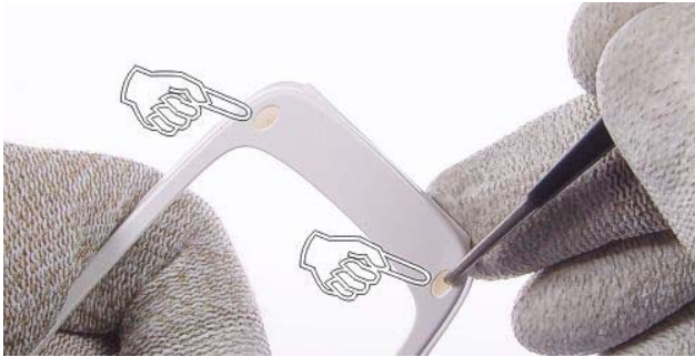
21.) Push out the C-Cover Rubber Spacer with tweezers.
