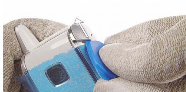
6.) Use the SRT-6 to open the clip of the Antenna Cover .
