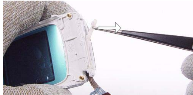
24.) Remove the Flap Stop with tweezers if necessary.
