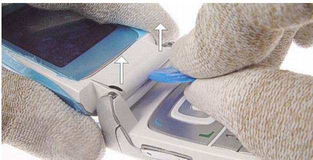
3.) The B-Cover Bezel is glued to the B-Cover . Use the SRT-6 as a lever to lift it a bit.
