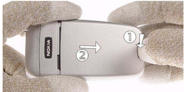
2.) Press the Release Button and remove the E-Cover .
