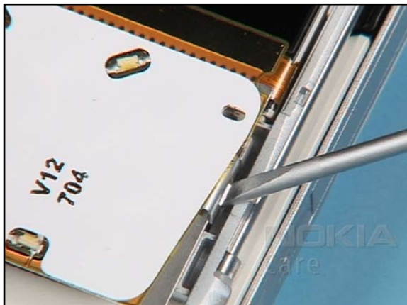
15. Open the metal latches of the SHIELD...
