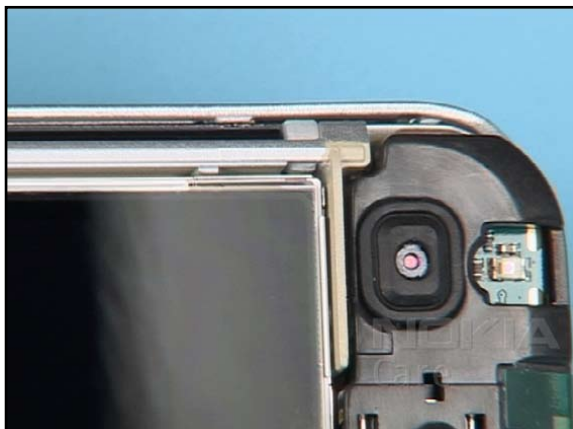
13. Do not forget placing the CAMERA DUST SHIELD.
