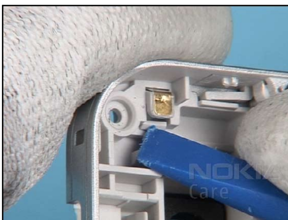
24. Release the clip of the BT ASSEMBLY.
