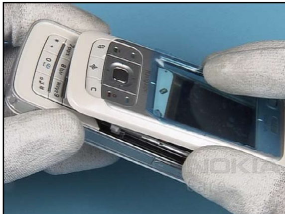
10. Shift it to bottom side direction and lift it up.
