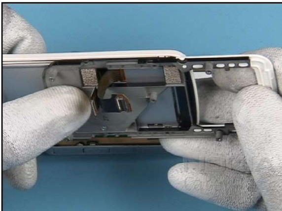
13. Slide the assembly into the open - position to gain the maximum flex foil lengths.
