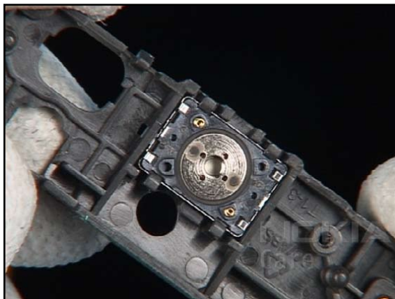
14. The EARPIECE is not glued in and can be replaced easily.
