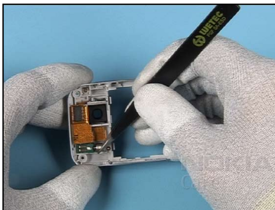
20. The removal of the VIBRA is easy.
