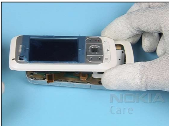
15. Carefully close the assembly and hold it into the middle position to gain the maximum flex foil lengths of the second connector.
