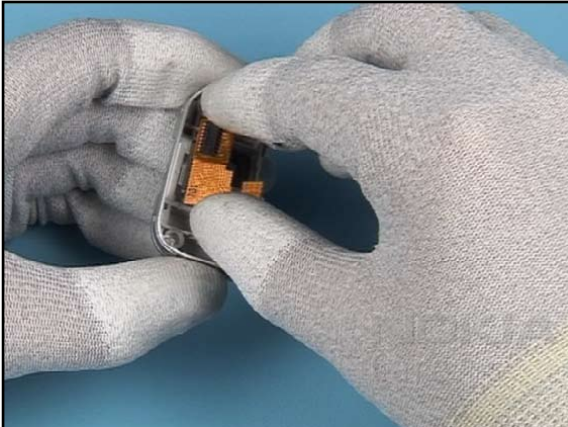
3. Fit the connector with LB FLEX MODULE into the B-COVER.
