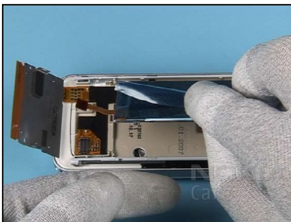
4. Position the LCD into its compartment.
