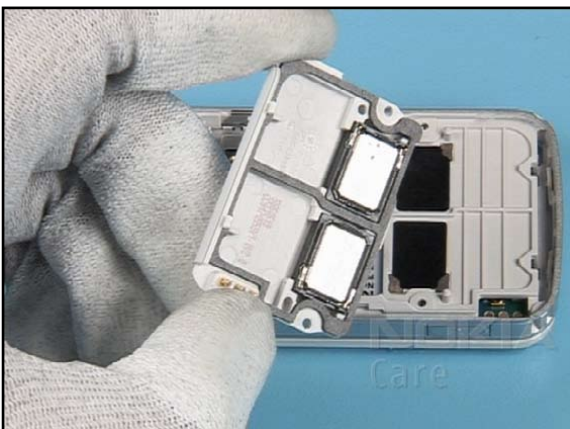
11. Both IHF SPEAKER can be removed, but fit them with new gaskets before reassemble.
