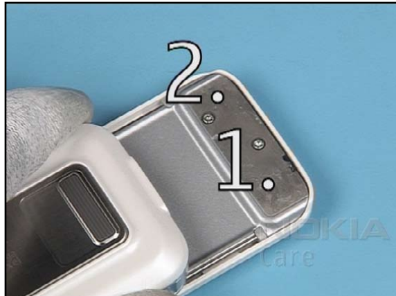
8. Unscrew both screws. It is not necessary to remove the 2nd screw if only A-COVER or FUNCTIONAL KEYMAT needs to be replaced.
