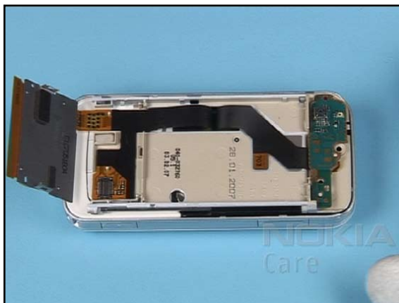
2. Mind the correct positioning when replacing the UI FLEX foils.
