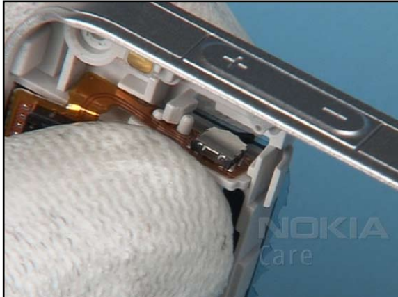
4. Position the switch as shown.
