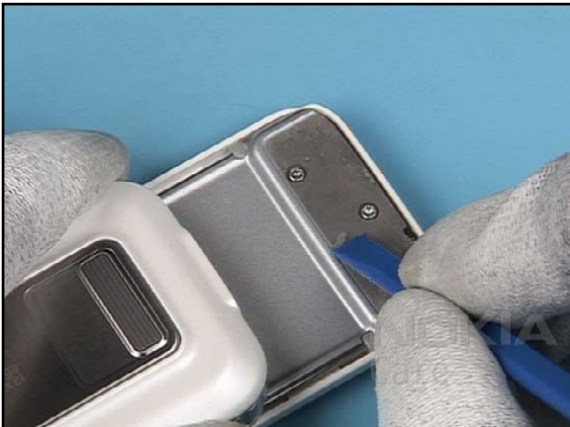
7. Remove the adhesive residues before reassembly.
