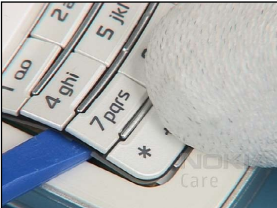
27. While inserting the KEYMAT - use the SS-93 only. Mind the components underneath.
